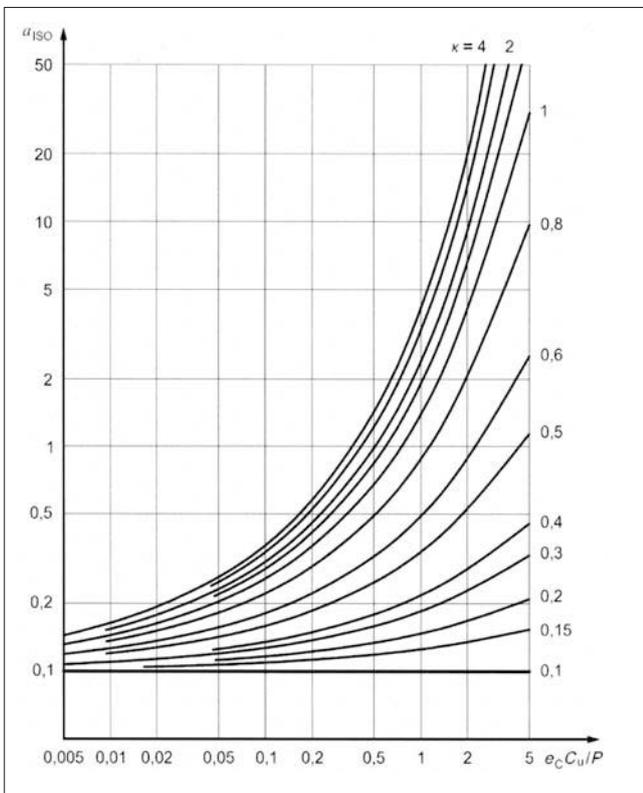
Figure A.5 Life modification factor  $a_{ISO}$  (thrust roller bearing)
