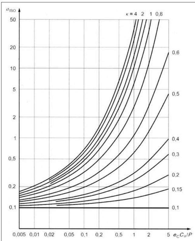
Figure A.3 Life modification factor  $a_{ISO}$  (radial roller bearing)
