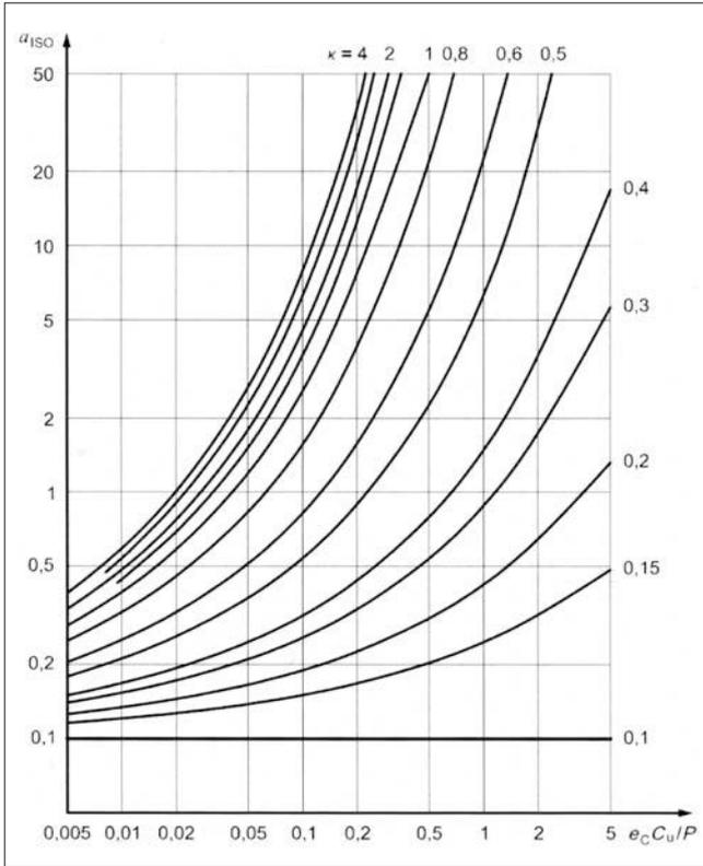
Figure A.2 Life modification factor  $a_{ISO}$  (radial ball bearing)
