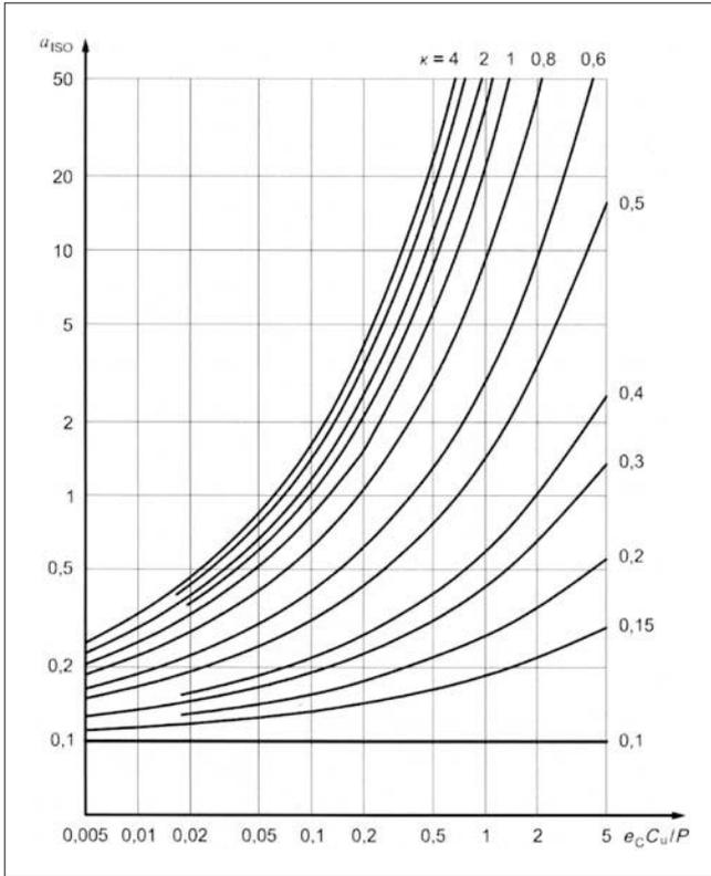
Figure A.4 Life modification factor  $a_{ISO}$  (thrust ball bearing)
