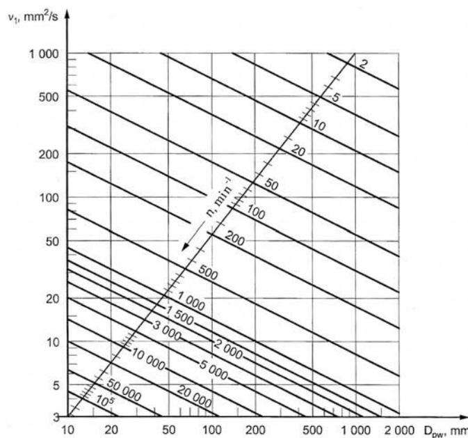
**Figure A.1 Reference kinematic viscosity  $\nu_1$**
