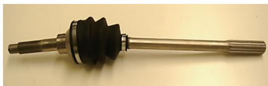
**Fig. 5** Exterior of CVJ mounted on Suzulight Van FE
