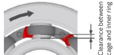
Movement of grease to the outer diameter side of the inner ring is suppressed and flow to the outside is prevented by optimizing clearance between the cage and inner ring.
