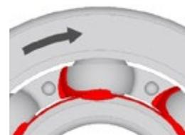
Grease scraped from the ball surface by the cage may accumulate on the inner diameter surface of the cage, move to the outer diameter surface of the inner ring, continue on to the seal groove, and flow to the outside.
