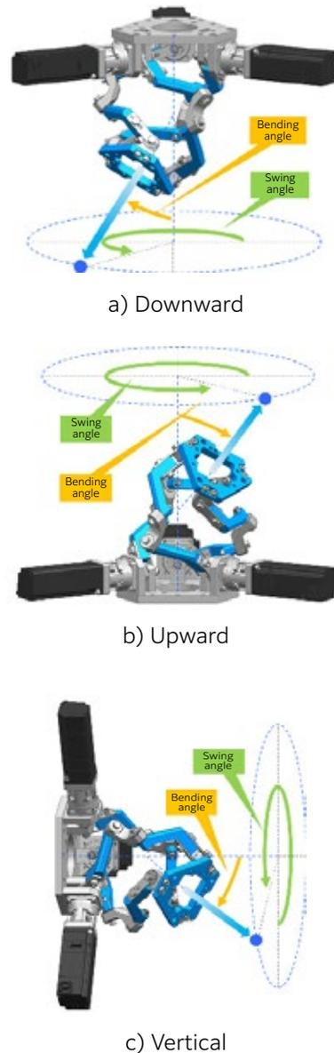
**Fig. 10** Installation direction
