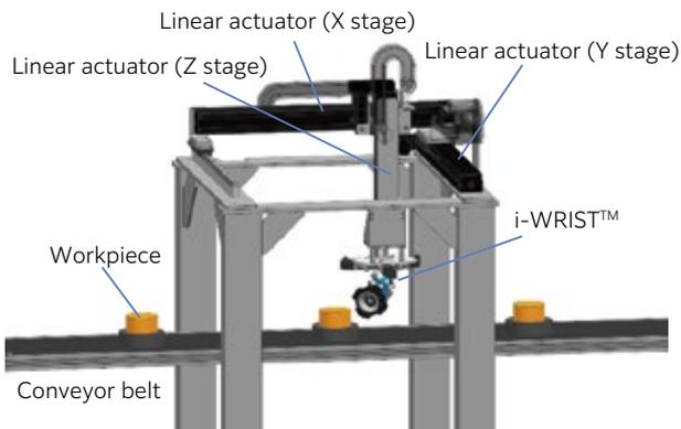
**Fig. 9** Configuration example of in-line system
