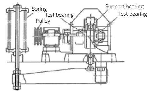
**Fig. 6** Schematic drawing of the life test rig
