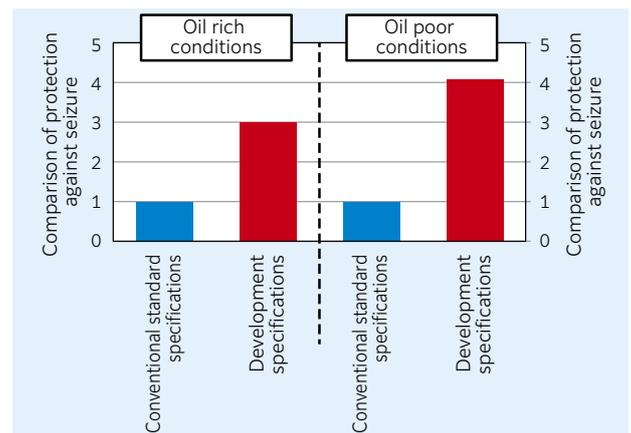
**Fig. 4** Seizure resistance evaluation results for development specification roller end face radius (Comparison result when the seizure resistance of the conventional standard specification is set to 1)
