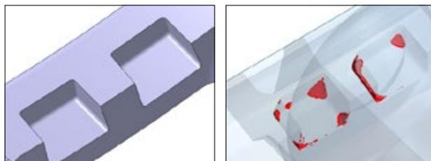
(a) Cage concave shape (same view as **Fig. 3** (b)) (b) Lubricant flow analysis results (red parts: lubricant) (bearing shown as semi-transparent)
