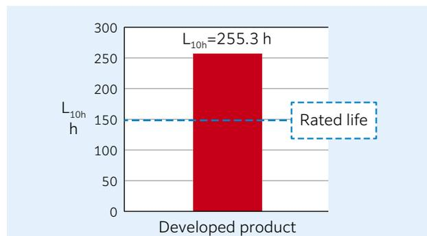
Fig. 7 Life test results under contamination lubrication condition
