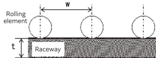
**Fig. 2** Thickness of bearing ring and rolling elements
