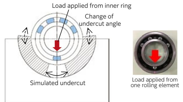
Fig. 8 Outer ring crack tester
