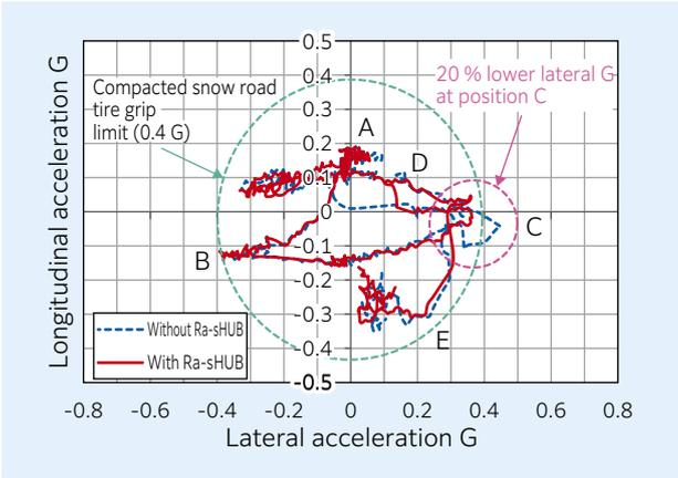
**Fig. 15** Test results (Longitudinal acc, Lateral acc)
