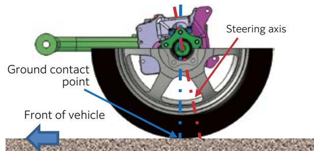
**Fig. 3** Layout of rear wheel with Ra-sHUB
