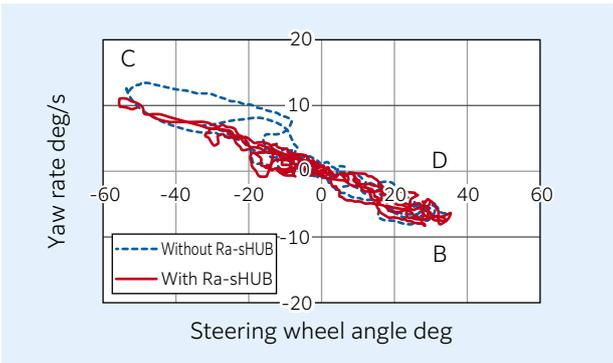
**Fig. 16** Test results (Steering angle, Yaw rate)
