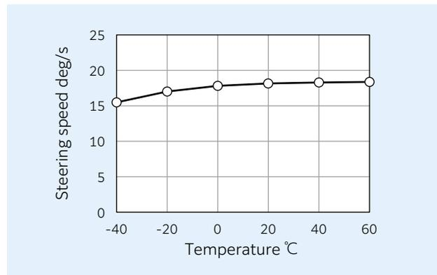
**Fig. 9** Relations of temperature and steering speed
