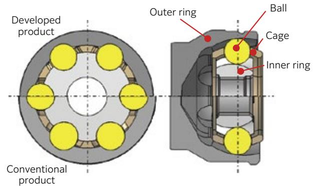
**Fig. 3** Comparison of outer dia. and axial length
