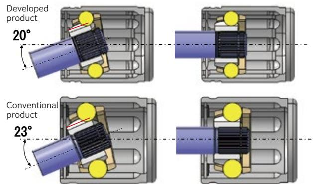
**Fig. 6** Comparison of ball groove length (red line)
