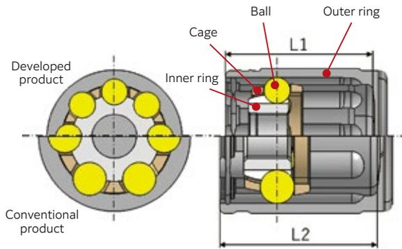
Fig. 8 Comparison of outer dia. and axial length
