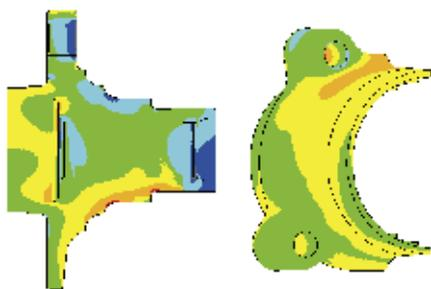
Fig. 8 FEM analysis sample of axle bearing
