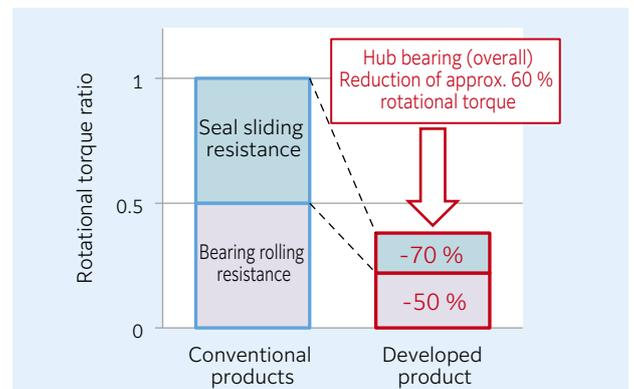
**Fig. 5** Performance of Low Friction Hub Bearing III
