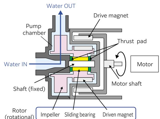
**Fig. 5** Structure of magnetic drive electric water pump
