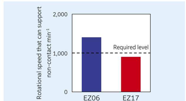
**Fig. 4** Test result of contact of shaft and BEARPHITE (Shaft outer diameter 2 mm)
