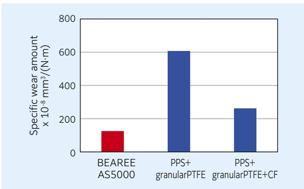
Fig. 10 Result of wear test of PPS
