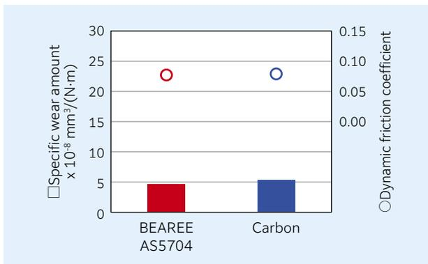
**Fig. 8** Results of friction and wear test of BEAREE AS5704 bearing and carbon bearing
