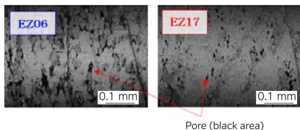
**Fig. 3** Enlarged photo of inner surface (Inner diameter 2 mm)
