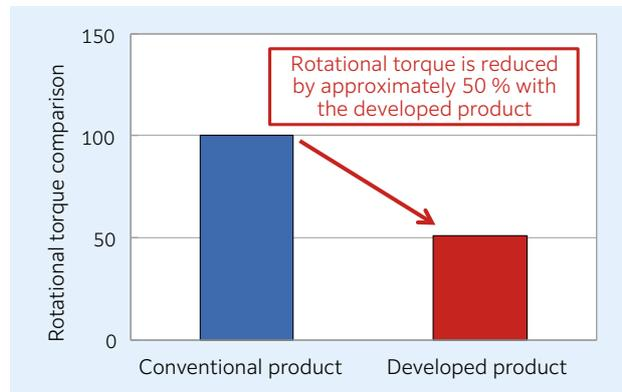
**Fig. 16** Torque test of the developed bearing
