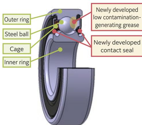
**Fig. 5** Low Contamination Generation Bearing for Servo Motors
