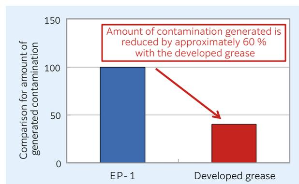
**Fig. 9** Contamination generation test of the developed grease\*
