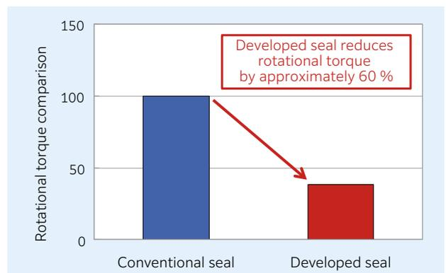
Fig. 13 Torque test of the developed seal
