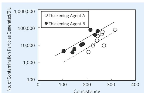
**Fig. 8** Relationship between grease consistency and contamination generation
