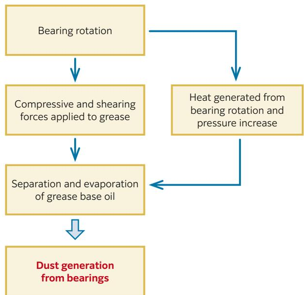
**Fig. 6** Dust generation from bearings
