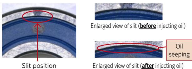
Fig. 11 Performance test of the seal slit
