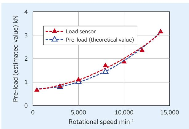
**Fig. 5** Test result of the bearing preload detection
