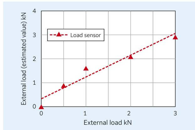
**Fig. 6** Test result of the external load detection
