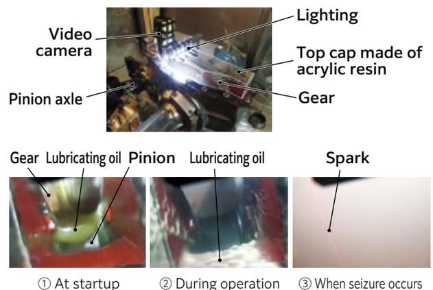
**Fig. 11** Internal state of driving-unit in low-temp. environment
