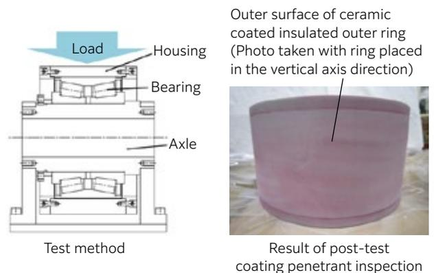
**Fig. 6** Strength test result of ceramic-insulation coating
