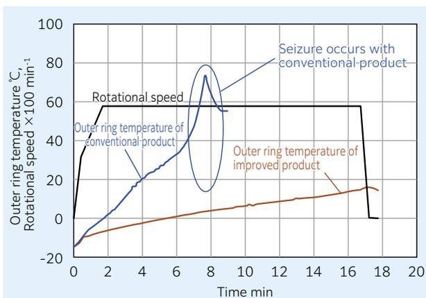
Fig. 13 Start-up test result in low-temp. environment
