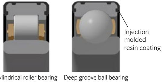
**Fig. 7** Resin-insulated bearing
