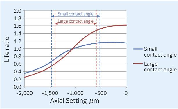
Fig. 18 Effect to bearing life for temperature change
