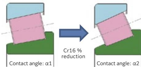
Wider axial cross section (aspect ratio 0.9)
