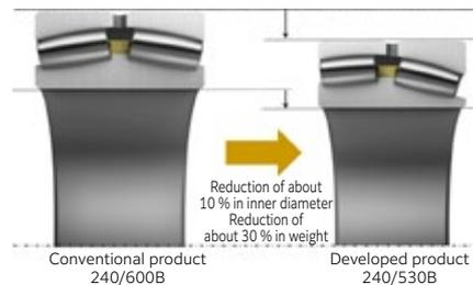
**Fig. 5** Example of design for downsizing
