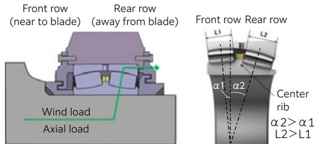
**Fig. 3** Loading condition **Fig. 4** Asymmetrical design
