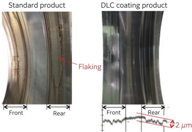
**Fig. 11** Test results with full scale bearings
