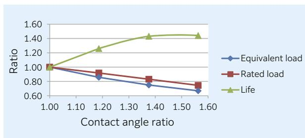
**Fig. 15** Example 1 Relationship between contact angle and bearing life for axial load side row
