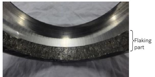
**Fig. 9** Outer ring raceway after 300 hours
