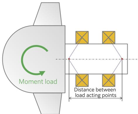
**Fig. 14** Relationship between applied load and bearing span
