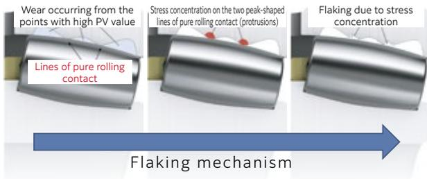
**Fig. 6** Damage mechanism
