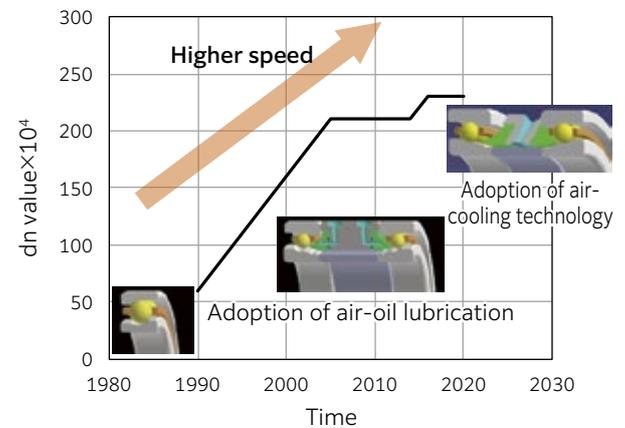
**Fig. 2** Transition into higher speed machine tool bearings
