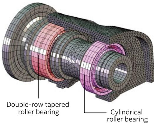
**Fig. 4** Analysis model of wind turbine main shaft system
