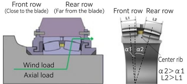
**Fig. 5** Left: Loading condition, Right: Asymmetrical design
