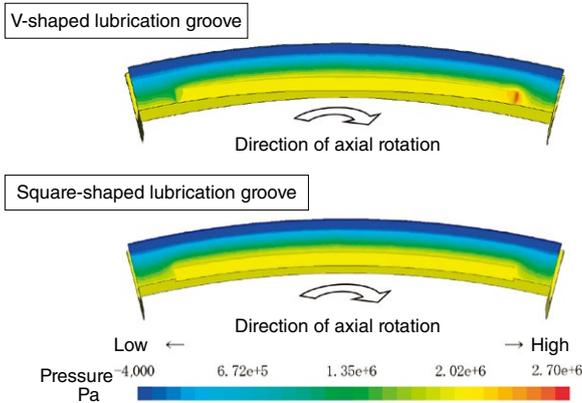
Fig. 5 Oil film pressure distribution on sliding surface
