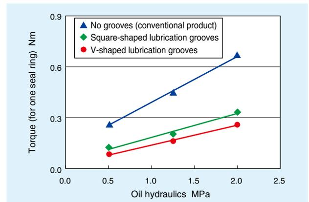
Fig. 4 Relationship between oil hydraulics and torque
