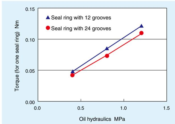
Fig. 11 Relationship between oil hydraulics and torque
