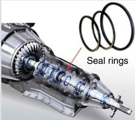
In order to achieve demands of fuel consumption standard, seal rings for automotive transmission are required to further reduce torque and oil leak. NTN developed “Low Torque Seal Ring” and started mass production. It has V-shaped lubrication grooves, which reduces torque by 60% in comparison with conventional products. This article introduces fluid analysis results of torque reduction by V-shaped lubrication grooves in “Low Torque Seal Ring”.
