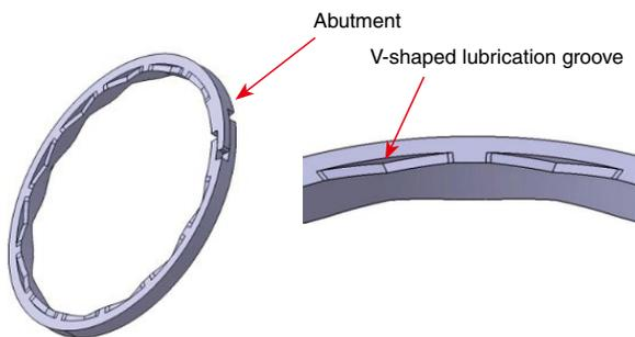
Fig. 1 Low torque seal ring
