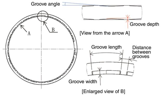
Fig. 6 Analysis of seal ring (24 grooves)
