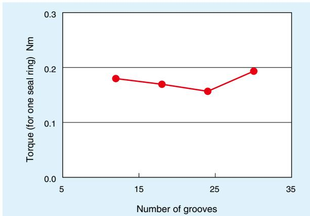
**Fig. 8** Relationship between number of grooves and torque
