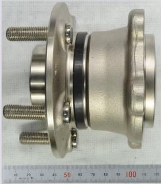
The Fuel efficiency regulations have been strengthening, therefore the good fuel efficiency is one of the important requirements from the field. Based on this background, **NTN** has been developing the low friction Hub Bearing continuously. The Low Friction Hub bearing III applicable to such around 60% low torque requirement is introduced in this report.
