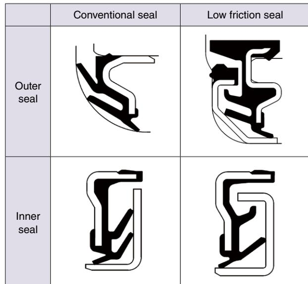
**Fig. 6** Structure of conventional seal and low friction seal
