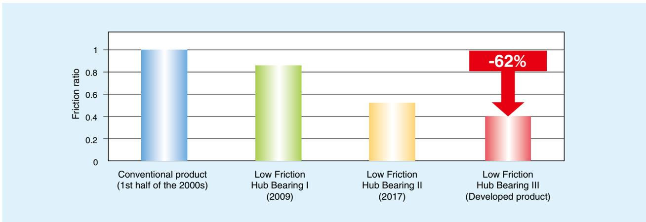
**Fig. 3** Transition of development for torque reduction
