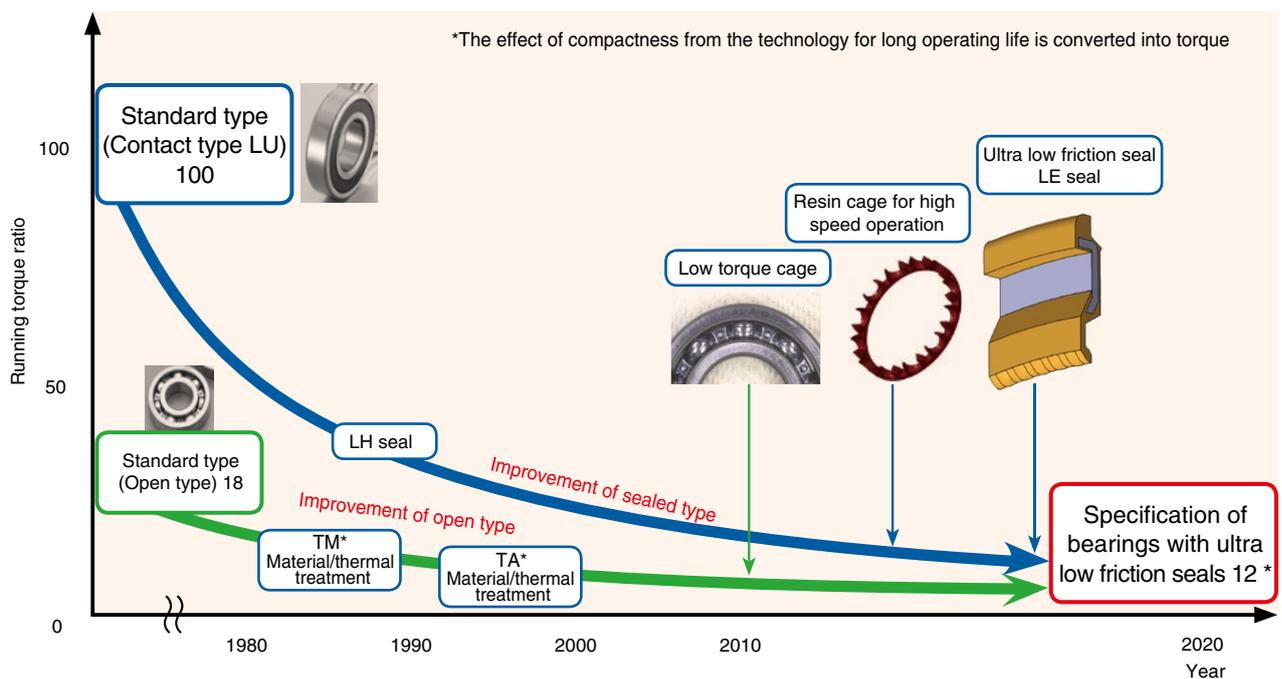
**Fig. 2** Transition of development of deep groove ball bearings<sup>2)</sup>
