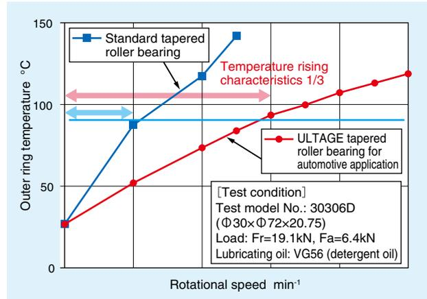
**Fig. 10** Seizure resistance test (temperature rising test)
