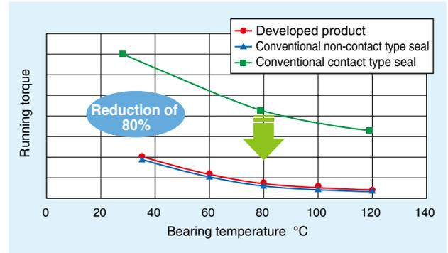
Fig. 6 Relation between bearing temperature and running torque
