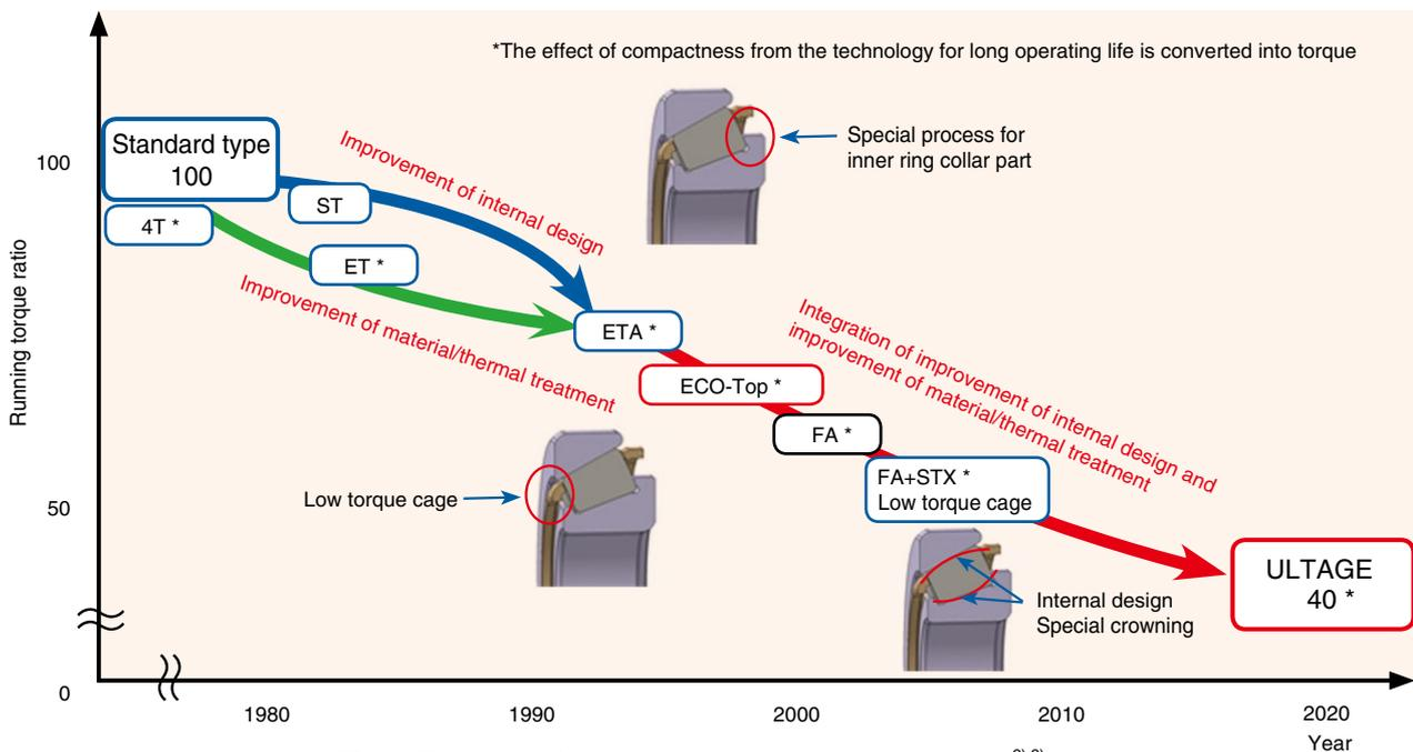
Fig. 4 Transition of development of tapered roller bearing<sup>2),3)</sup>
