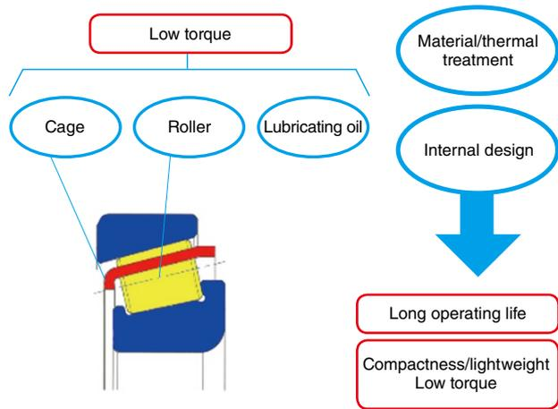
Fig. 3 Tapered roller bearing and characteristics
