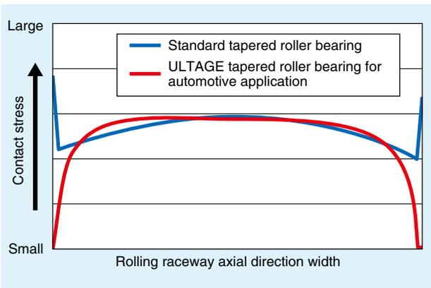
**Fig. 8** Contact stress distribution on the raceway
