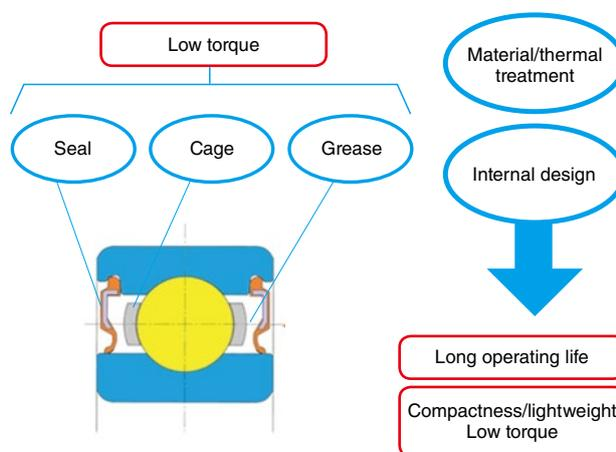
**Fig. 1** Deep groove ball bearing and characteristics
