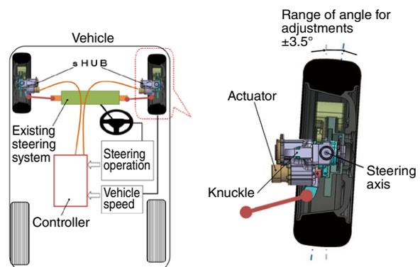
Fig. 1 Vehicle with sHUB installed (on front wheels)
