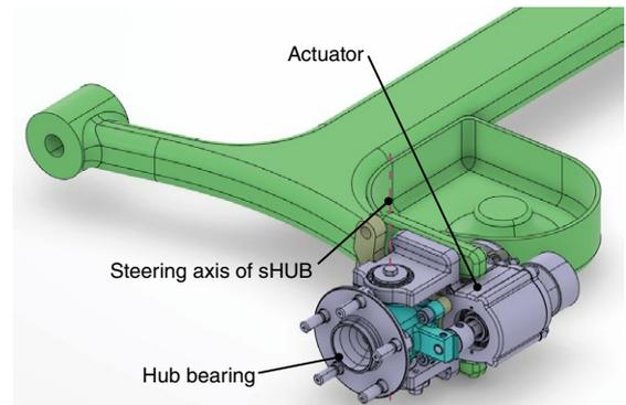
**Fig. 5** sHUB installed on rear wheel
