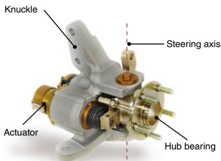
**Fig. 2** Prototype of sHUB
