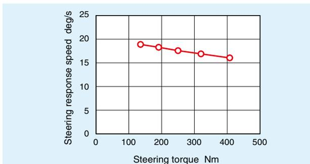
**Fig. 9** Relationship between steering torque and steering response speed
