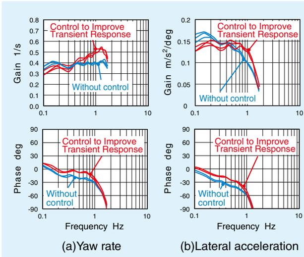
Fig. 11 Test result of frequency response characteristics
