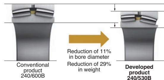
Fig. 11 Example of design for down sizing
