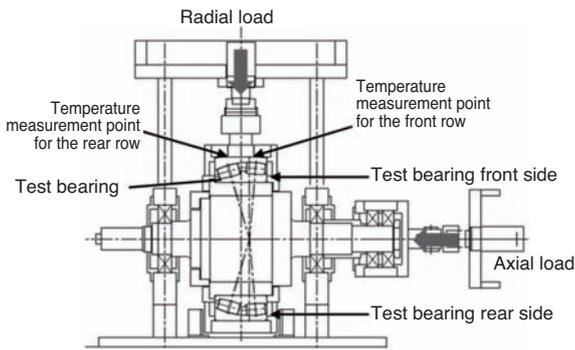
Fig. 12 Testing machine for actual size bearings test
