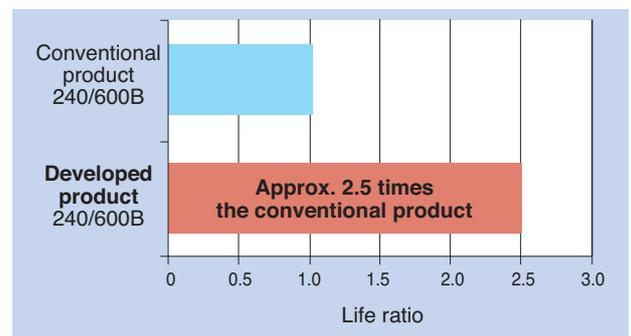
Fig. 9 Comparison result of calculation life of conventional SRB and asymmetrical SRB
