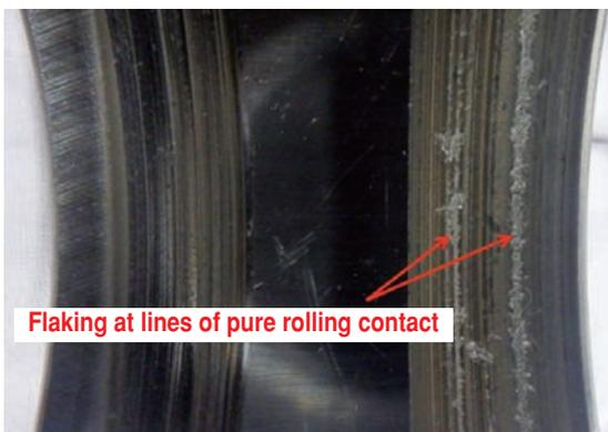
Fig. 6 Flaking on non-slip line
