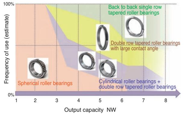
Fig. 3 Relationship between generation capacity and type of main shaft bearings<sup>2)</sup>
