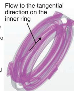
**Fig. 10 (b)** Cooling air flow of development designed spacer (Fluid analysis results)
