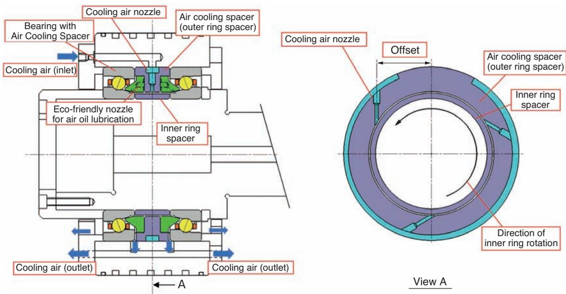
Fig. 1 Machine tool main spindle bearings with air cooling spacer (for air oil lubrication)<sup>1)</sup>
