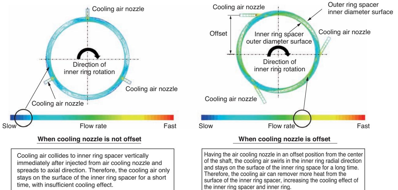
Fig. 2 Cooling air flow between inner and outer spacers (Fluid analysis results)<sup>1)</sup>
