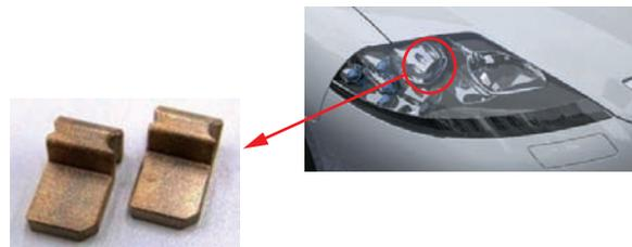
**Fig. 11** Self-lubricating sliding material (For AFS)
