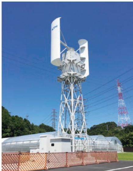
Fig. 13 10kW vertical axis wind turbine
