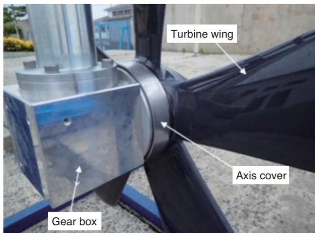
**Fig. 14** Cover of blade axis
