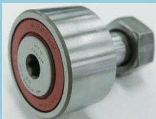
Cam follower is used for guide rail, index machine and so on. In these mechanisms, cam follower is often mounted outside exposing position. Therefore cam follower might be exposed to fluid such as cutting oil, and improvement of seal performance to prevent grease leakage is needed.
