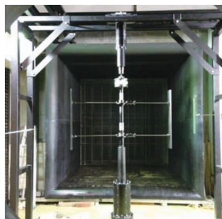
Fig. 16 Wind tunnel experiment of vertical axis wind turbine (Mie University Large Wind Tunnel)
