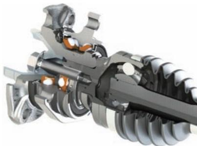
Compare to a standard solution, the mass of the wheel hub & CVJ assembly is reduced by 21.2%, with 18.2% by PCS & 3% by aluminum centering.
