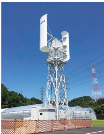
Fig. 13 10kW vertical axis wind turbine
