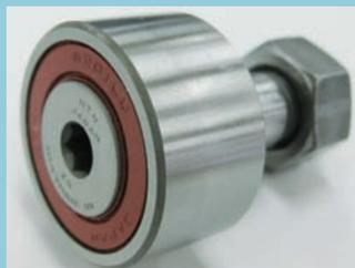
Cam follower is used for guide rail, index machine and so on. In these mechanisms, cam follower is often mounted outside exposing position. Therefore cam follower might be exposed to fluid such as cutting oil, and improvement of seal performance to prevent grease leakage is needed.
