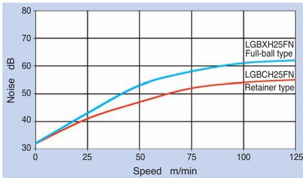
Fig. 6 Noise level of linear guides
