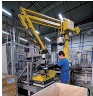
Example of cobot to follow man's movements while multiplying its strength
