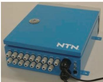
Fig. 1 Data acquisition module, Wind Doctor®
