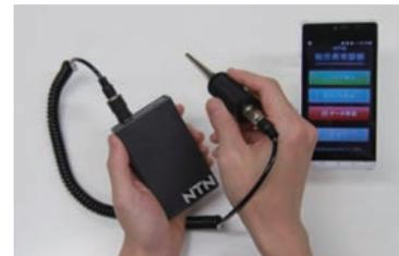
Fig. 8 Handy type failure detection device
