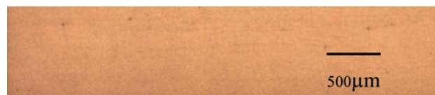
Fig.10 Cross sectional microstructure of laser formed Ti compact
