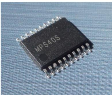
Fig. 2 Appearance of MPS40S
