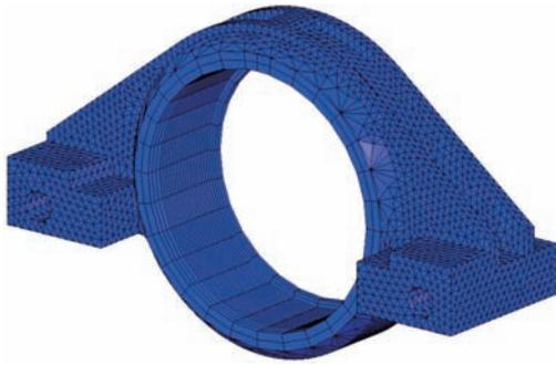
Fig. 6 Analytical model of housing for spherical roller bearing
