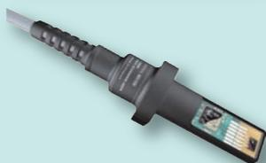
We present here a new linear magnetic sensing technology, based on Tunnel Magneto Resistance (TMR). The TMR principle derives from Spintronics, a new branch of Physics which received the 2007 Nobel Prize in Physics. Contrary to “traditional” electronics, a Magnetic Tunnel Junction (MTJ) uses not only the electric charge of the electron, but also its quantum spin value.
