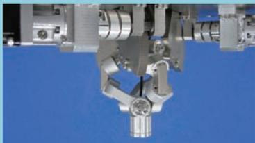
NTN has developed a Parallel link High speed Angle Control Equipment (PHACE) that can control the angle with two-degrees-of-freedom quickly and over a wide range (max bend angle : 90 deg.). Adapting the unique parallel link mechanism enables both compact size and wide operating range. In addition, by developing the drive
