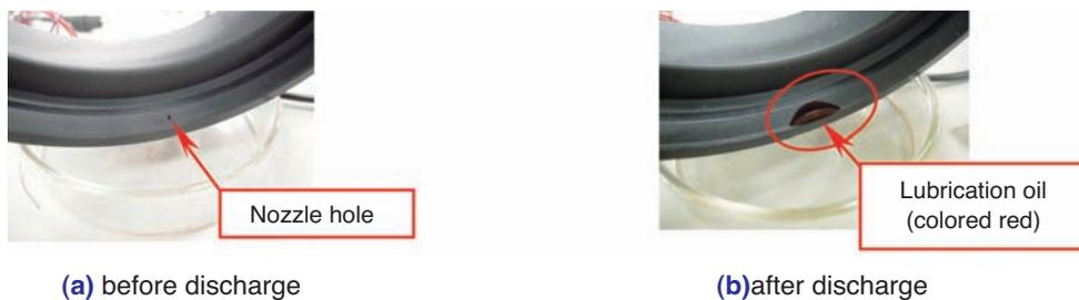
Fig. 3 Discharge of lubricating oil
