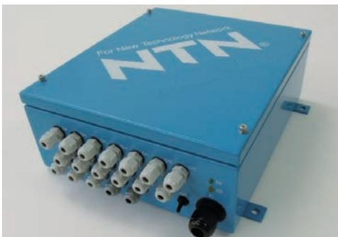
Fig. 2 Data acquisition module
