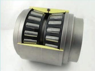
Journal bearings are very important components of railway vehicles as they directly affect the vehicle's running stability. Sealed type double row tapered roller bearings with grease packed are traditionally used as journal bearings. The grease packed in the bearing has a tendency to move out from contact surface of raceways. Good oil providing capability of a grease to the raceways of a bearing is an important factor for the grease life.
