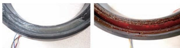
(a) Before lubricating oil discharge (b) After lubricating oil discharge
