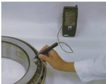
Fig. 6 IC Tag integrated bearing
