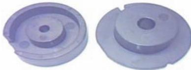
Amorphous core (a component of choke coil)
