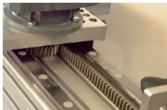
Fig. 11 Rack-and-pinion drive
