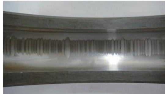
Fig. 7 Outer raceway failure by electrical pitting
