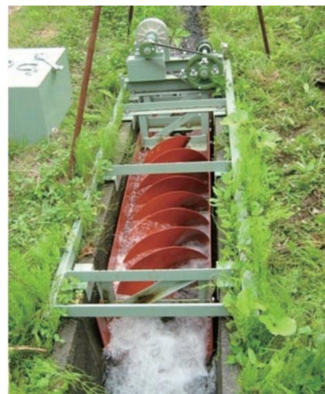
**Fig.6** Power generation system using axial type turbine set in a small irrigation canal
