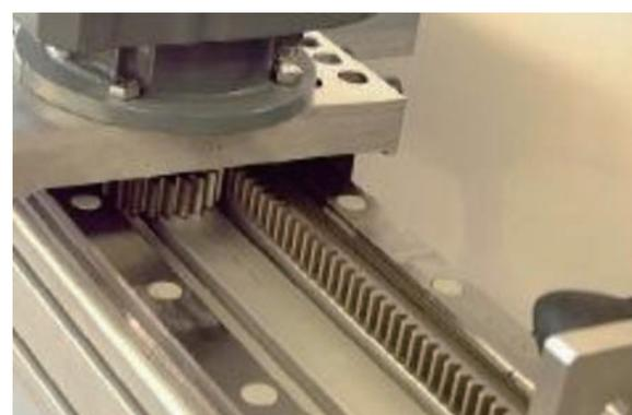
**Fig. 11** Rack-and-pinion drive
