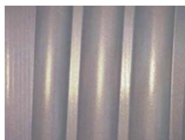
**Fig. 4** Appearance of thread groove on nut
