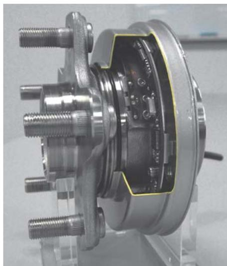
Fig. 1 Load sensor-integrated hub bearing
