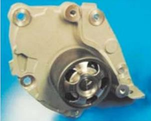
Water pumps used on automobile engines are used to circulate the coolant between the engine and heat exchangers. Water pumps are very important to the operation of the engine and require a high level of reliability. The seals and bearings inside the water pump are critical components and require the same high level of reliability.
