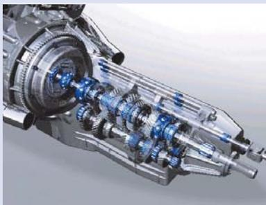
There are demands to improve the torque, size, weight, life and rigidity of rolling bearings used in automotive transmissions and differentials.
