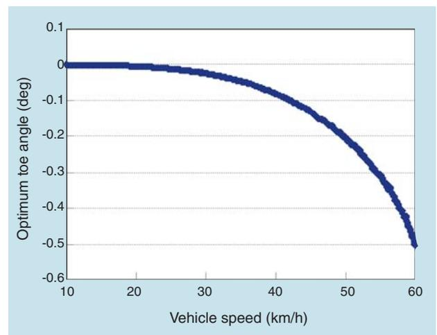
Fig. 17 Optimum toe angles for vehicle speeds
