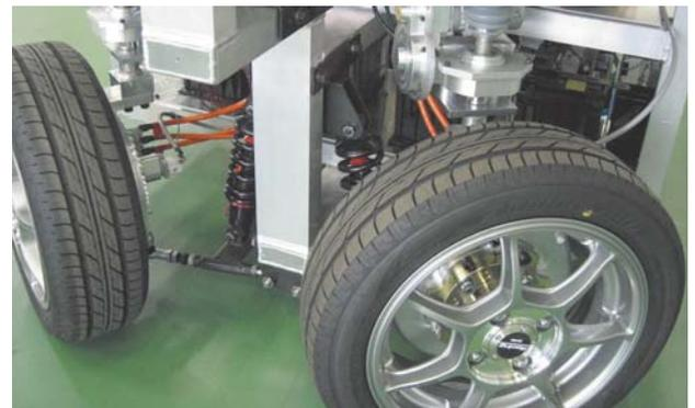
**Fig. 7** Steering in pivot-turning mode
