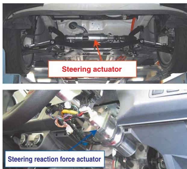
Fig. 11 View of NTN-SBW mounted in test vehicle
