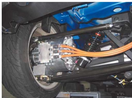
Fig. 9 IWM mounted in a vehicle (on the rear left wheel)
