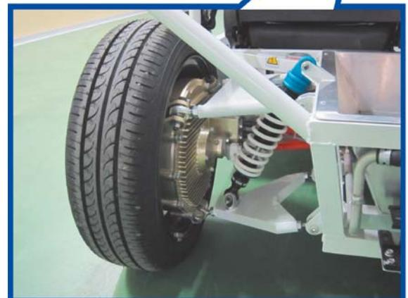
**Fig. 4** Test EV (above) and mounted in-wheel motor (below)
