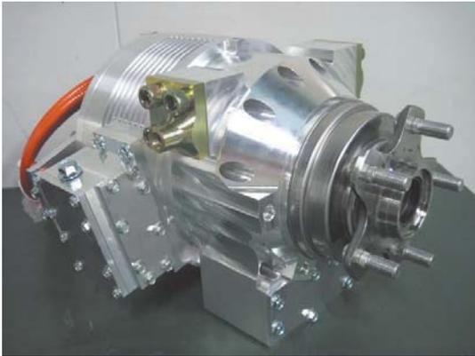
**Fig. 1** Appearance of in-wheel motor
