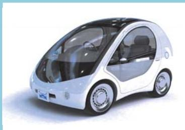
NTN has developed an In-wheel Motor System for commuter vehicles that could become a stepping stone that promotes the spread of electric vehicles (EV). The in-wheel motor unit that was developed can be installed in 14-inch wheels. In the test EV, it was shown that space in the car was able to be utilized effectively. This paper introduces the In-wheel Motor system that was developed and the test EV.
