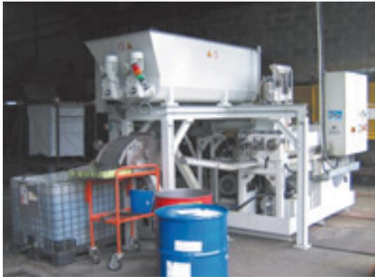
Fig. 15 Grinding sludge briquetter
