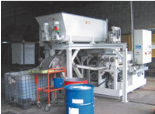
Fig. 15 Grinding sludge briquetter
