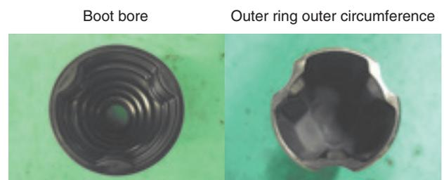
Fig. 6 Shape of TJ boot bore and outer ring O.D.
