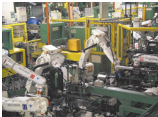
Fig. 9 CVJ robot assembly line
