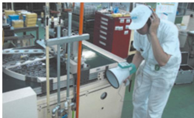
Fig. 9 Check by air leak detector
