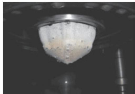
**Fig. 2** The film situation of the Punch for the Outer Race Joint
