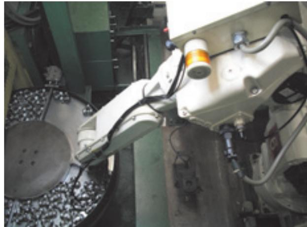
**Fig. 3** Intelligent parts supply device
