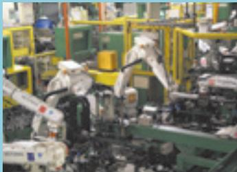
Human sense and experience are necessary for assembling processes. Therefore, automation (mechanization) has been difficult. We used sensor, robot, and simulation technologies, which have made remarkable advances in recent years, and succeeded in improving working environments in the assembly process for constant velocity joints (CVJ).
