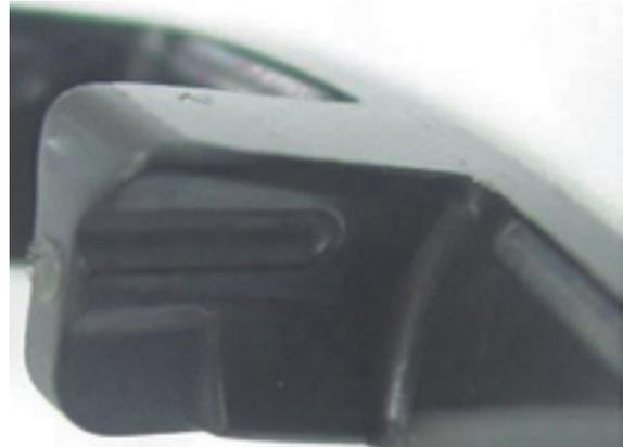
**Photo. 2** Condition of cage after 2000 (h) of rapid acceleration and slowdown test
