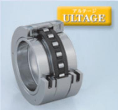
NTN has developed an angular contact ball bearing with minimum quantity and cooling jet (MQCJ) lubrication. A new jet lubrication method with an inner ring cooling system and an optimally minimized quantity lubrication mechanism for the raceway were adopted. A new product that has applied MQCJ lubrication to a single row cylindrical roller bearings was developed. We introduce this single row cylindrical roller bearing with the new jet (MQCJ) lubrication method.
