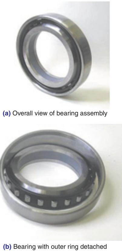
Fig. 10 Prototype of developed bearing
