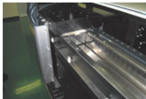
**Fig. 3** Linear Servomotor with iron core
