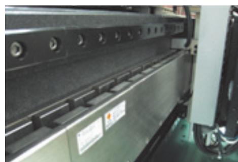
**Fig. 4** Coreless Linear Servomotor
