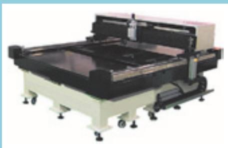
NTN has deeply cultivated precision positioning technology and applied it to various types of positioning systems. One of their major fields of application is LCD manufacturing equipment, and NTN provides large, long-stroke XY tables suitable for various types of equipment, including NTN LCD repair systems.
