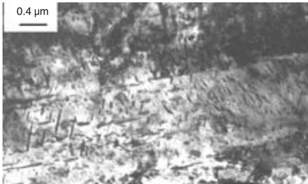
**Fig. 3** T.E.M micrograph of the structure after prior heat treatment
