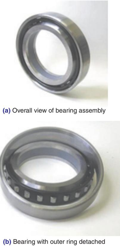
Fig. 10 Prototype of developed bearing
