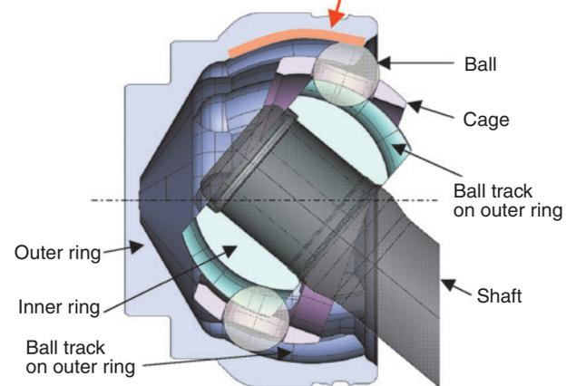
Fig. 3 Construction of EBJ at high-angle
