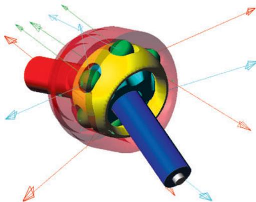
Red : Load working between outer ring track and balls
