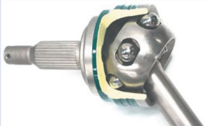
NTN Corporation has succeeded in developing a fixed-type constant velocity joint called TUJ that has the world's highest maximum operating angle –54 degrees–for automobile drive shafts. TUJ will allow four-wheel drive and front-wheel drive cars to have a greater steering angle, enabling a very small turning radius. This report summarizes the concept, design and characteristics of TUJ.
