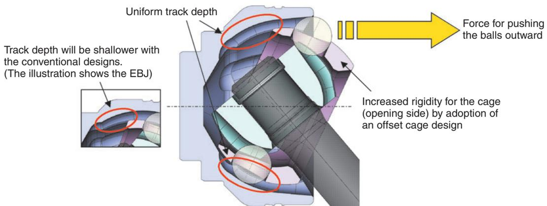
Fig. 6 Construction of TUJ at high angle
