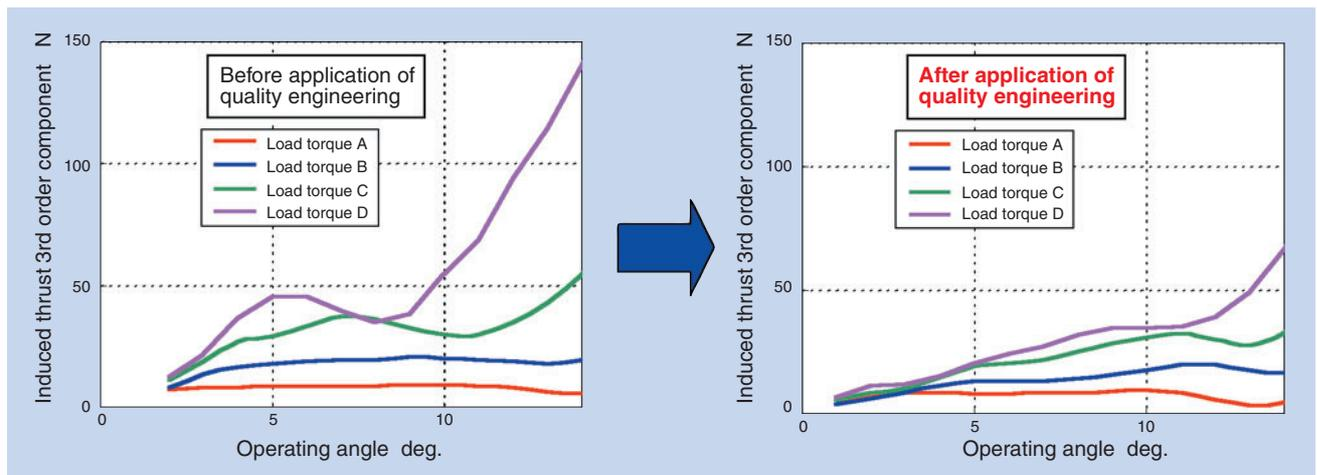
Fig. 7 Quality engineering for induced cyclic load reduction
