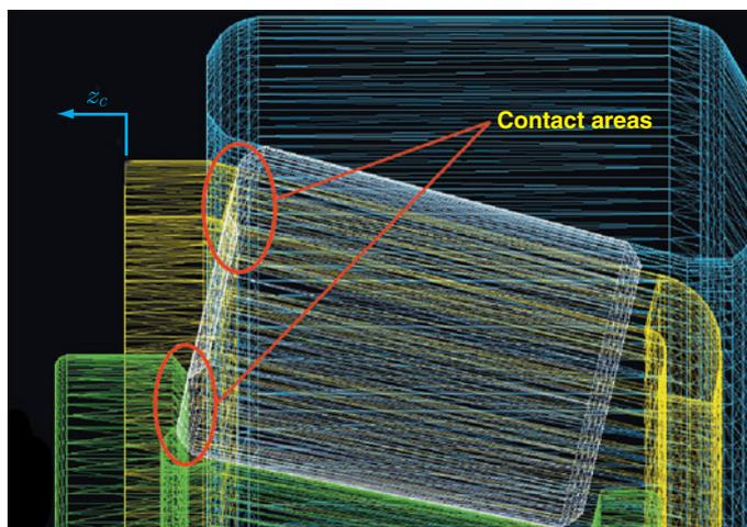
Fig. 12 Datum point for axial displacement of cage mass center
