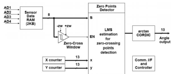
Fig. 7 Block diagram of the angle calculator
