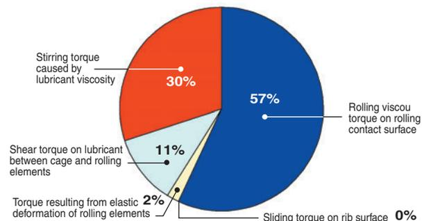
Fig. 10 Factors contributing to friction torque of tapered roller bearing used for pinion shaft support in near axle differential
