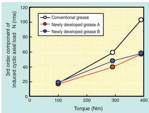
Fig.1 The 3rd order component of induced cyclic axial load of TJ
