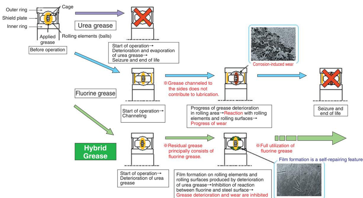
Fig. 4 Estimated mechanism for long grease life of Hybrid Grease
