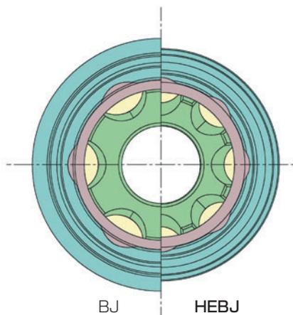
Fig. 2 Comparison of structure between BJ and HEBJ
