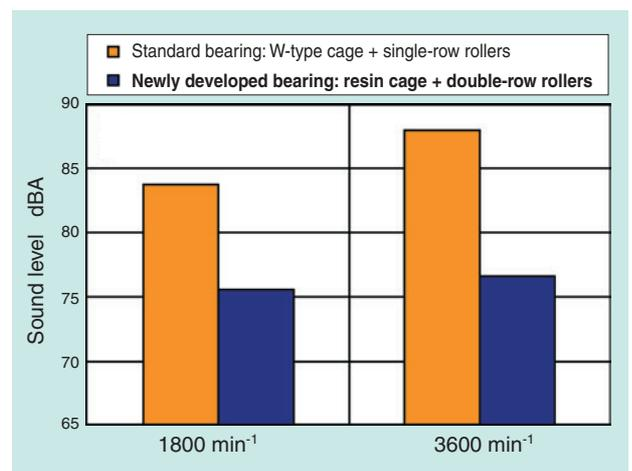
Fig 7 Measurement result of sound level
