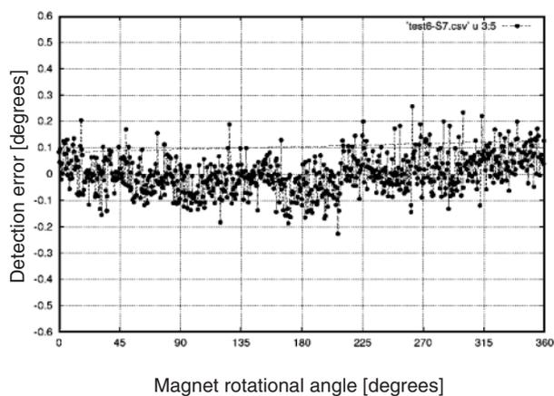
**Fig. 12** Angle detection result using a sensor bearing
