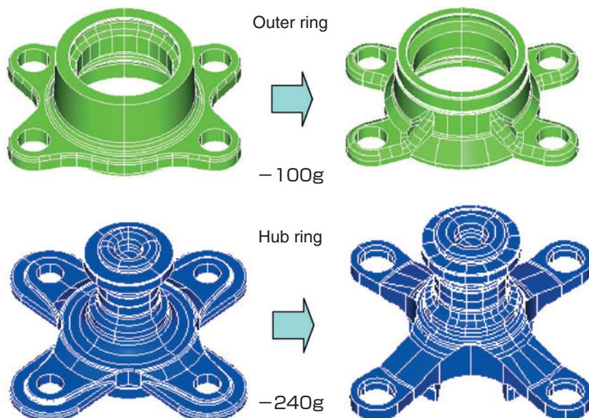
Fig. 10 Amount of each component Lightening
