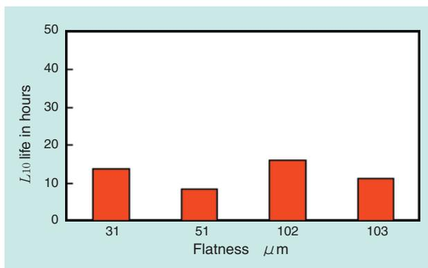
Fig. 4 Effect of race flatness on bearing life
