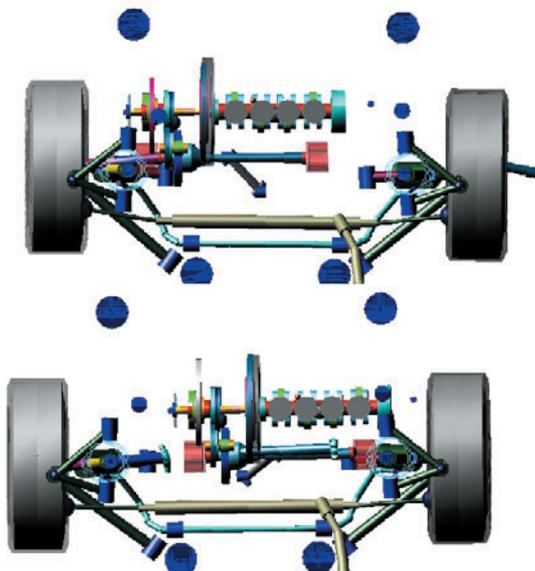
Fig. 6 Lateral engine mode shape (14.93Hz) of original model
