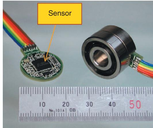
**Photo 2** Picture of a sensor bearing sample
