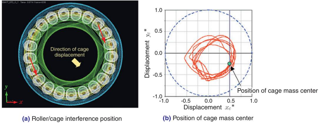
**Fig. 8** Relationship between the direction of cage displacement and cage/roller interaction position (standard cage)
