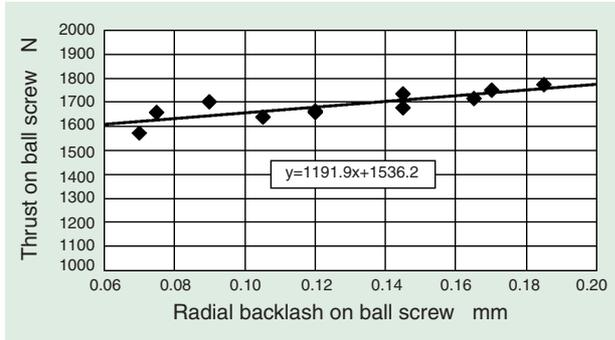
Fig. 4 Relationship between ballscrew's lash and thrust
