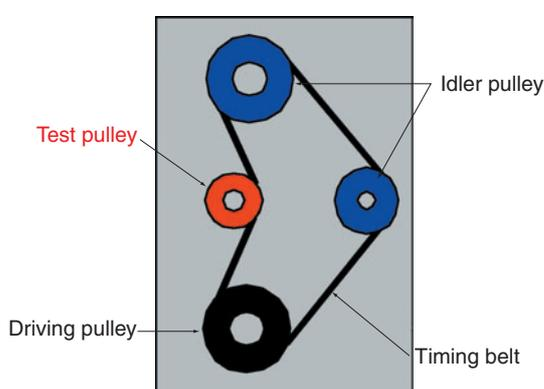
**Fig. 5** Tension pulley type test rig
