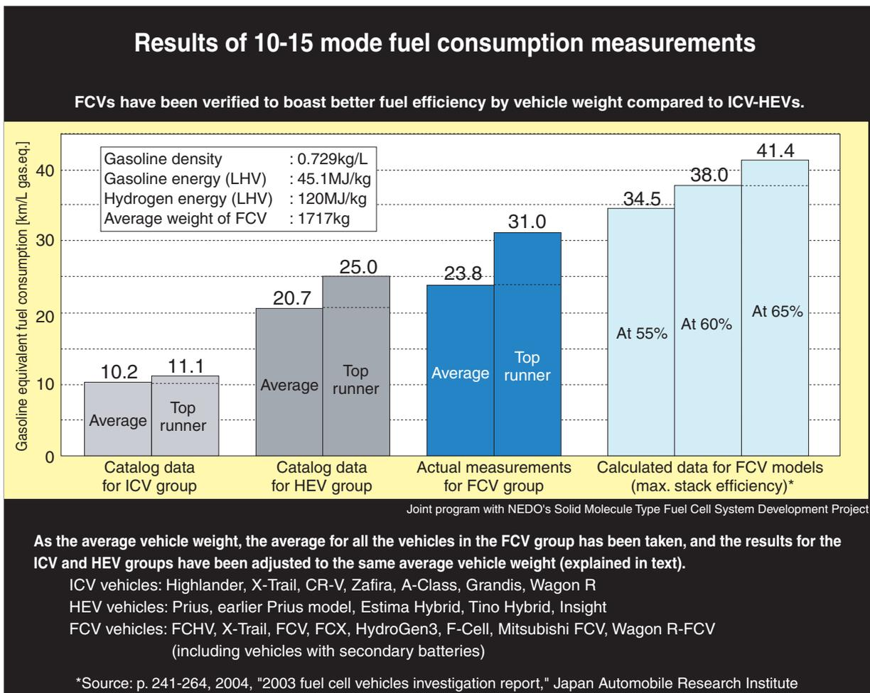
Fig.4 Japanese 10-15 mode fuel consumption on gasoline, hybrid and fuel cell vehicles (Home page of JHFC)
