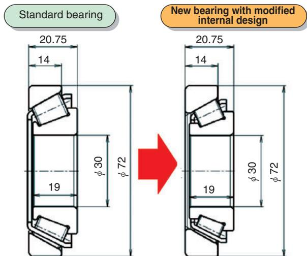
**Fig. 15** Comparison of bearing form
