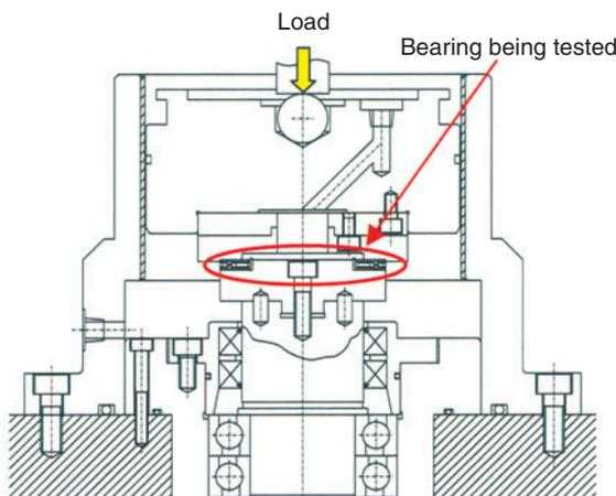
**Fig 1** NTN vertical type thrust bearing test rig
