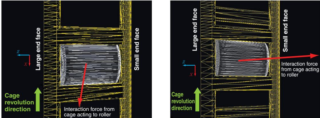
(a) Contact between roller rolling surface and cage pocket (b) Contact between roller large end and cage pocket
