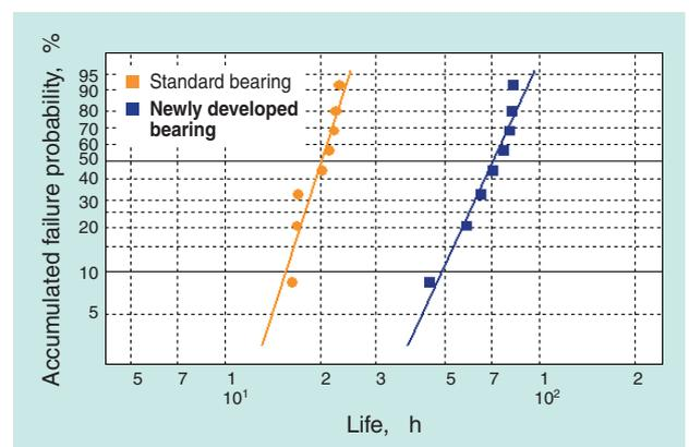
Fig 10 Result of life test for automatic transmissions
