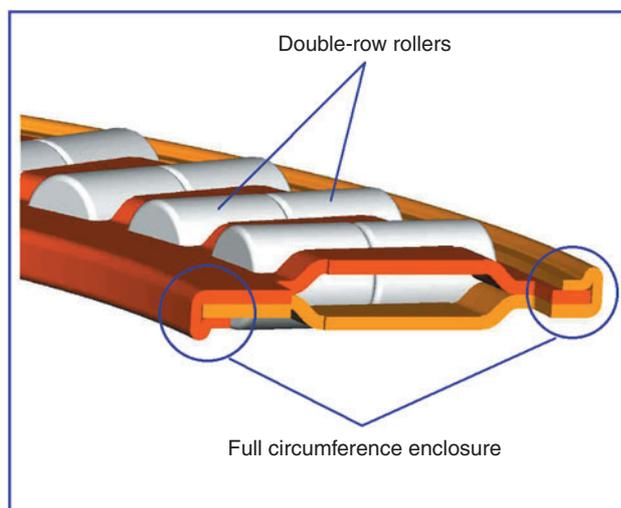
Photo 3 Double-row thrust needle roller bearings for automatic transmissions
