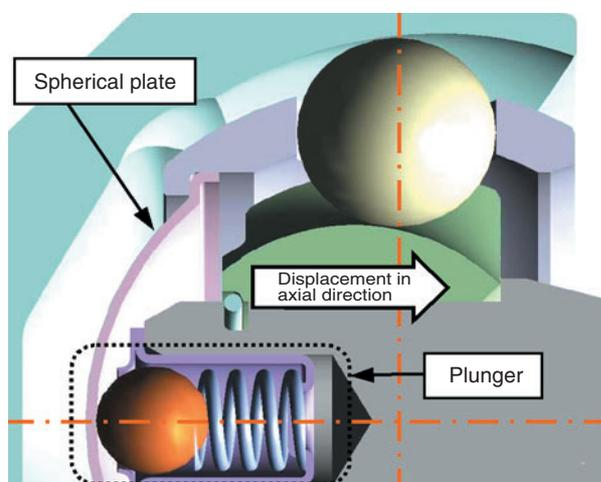
Fig. 2 Structure to reduce rotational play
