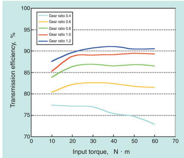
Fig. 7 Input torque and transmission efficiency (1000min<sup>-1</sup>)
