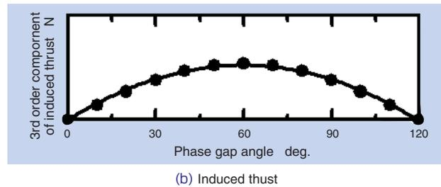
Fig. 11 Theoretical effect of CVJ phase gap on induced thrust
