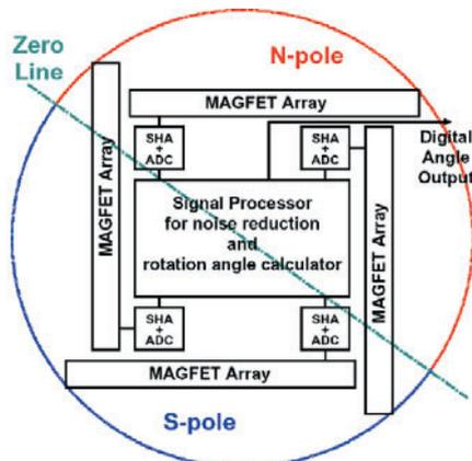
Fig. 2 Block diagram of the sensor chip
