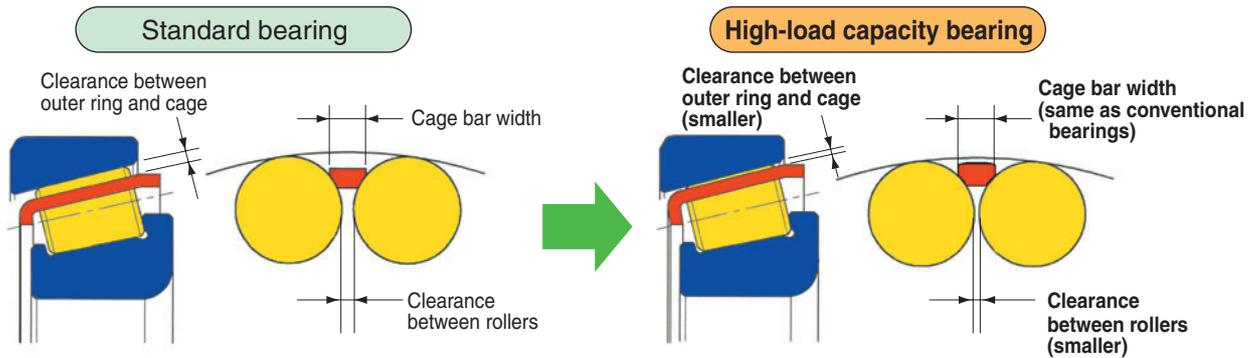
Fig. 1 Structure of high capacity tapered roller bearing
