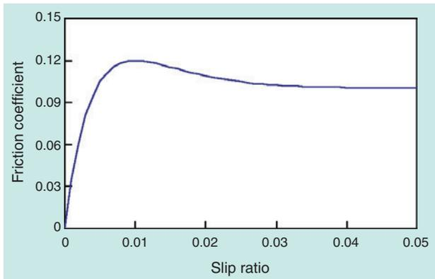
Fig. 2 Friction coefficient under boundary lubrication
