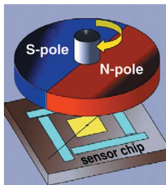
Fig. 1 Rotary encoder setup
