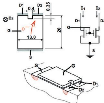
Fig. 3 Structure of MAGFET (unit  $\mu m$ )
