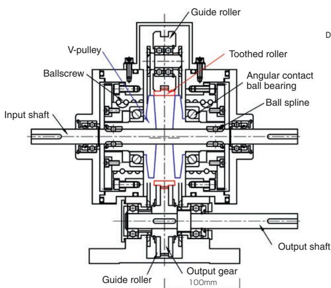
Fig. 1 Schematic view of MR-CVT
