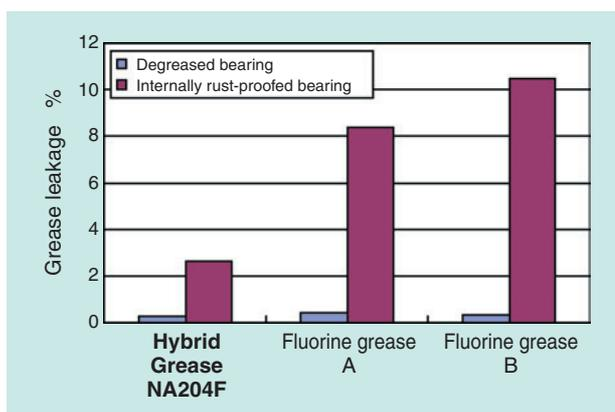
**Fig. 7** Leak rates of greases during rotation
