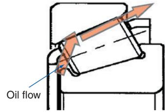
③ **Decrease in stirring torque caused by viscosity of lubricant**
