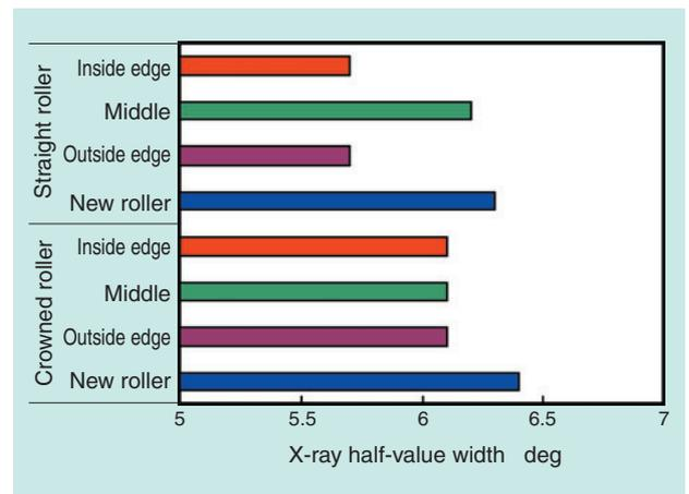
Fig. 8 X-ray half-value width of rolling marks on races
