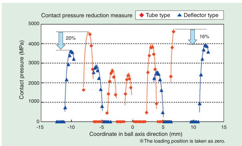
Fig. 3 Comparison of ball contact pressure
