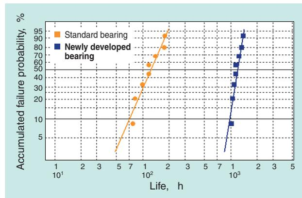
**Fig 4** Result of life test condition 2 with lean lubrication for car air conditioners
