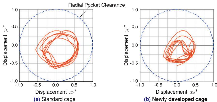
Fig. 7 Numerical results of cage mass center behavior in radial plane
