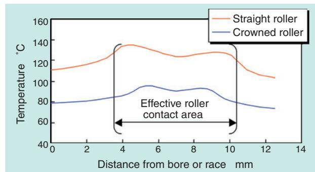
Fig. 16 Estimated temperature on raceway by FEM
