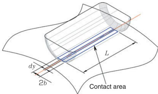
Fig. 11 Roller/race contact part
