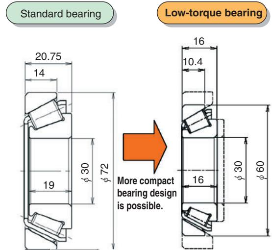
Fig. 18 Comparison of bearing size
