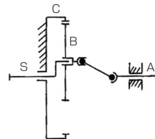
Fig. 3 Schematic of K-H-V type planetary gear
