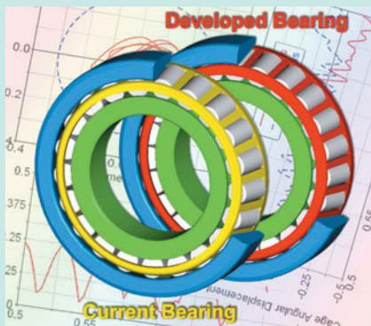
It is necessary to predict forces acting on a cage when designing rolling element bearings. It requires a dynamic simulation that can evaluate interaction forces between the bearing components including the cage as well as real-time behaviors of these components.
