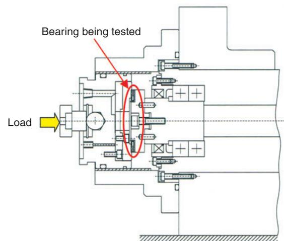
**Fig 2** NTN horizontal type thrust bearing test rig
