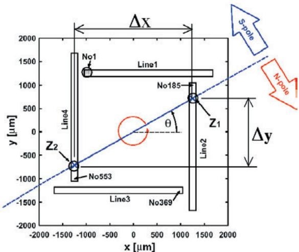
Fig. 4 Arrangement of sensor arrays (magnet is set at an angle  $\theta$ )
