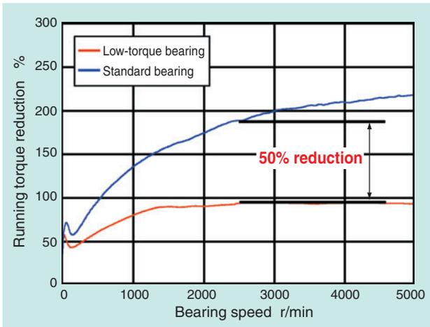
**Fig. 20** Relationship between speed and torque of current bearing and low torque bearing
