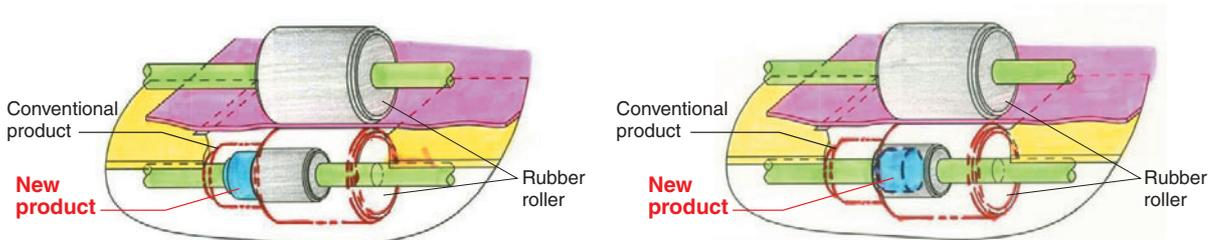
Rubber roller diameter can be made smaller and the axial direction more compact (red line shows a conventional torque limiter).
