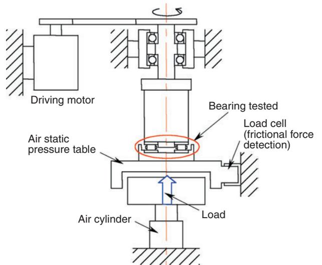
Fig. 12 NTN vertical type bearing frictional torque test rig
