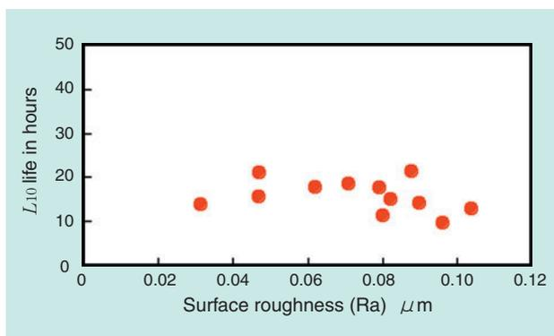
Fig. 3 Effect of race roughness on bearing life
