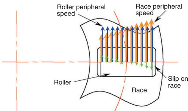
Fig. 10 Peripheral speeds and slip speed distribution in thrust needle roller bearing
