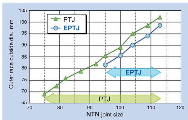
Fig. 2 Outer-diameter comparison between PTJ and EPTJ
