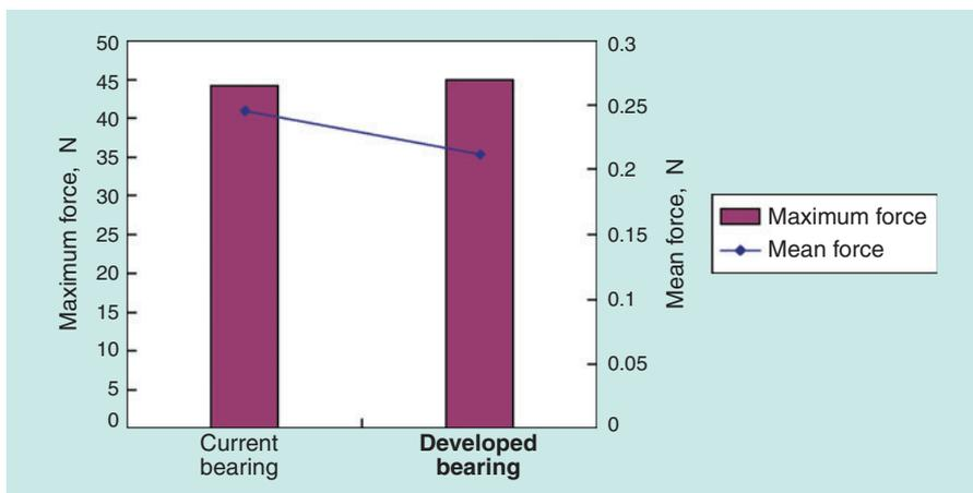
**Fig. 10** Mean value and the maximum value of cage/roller (rolling surface) interaction forces
