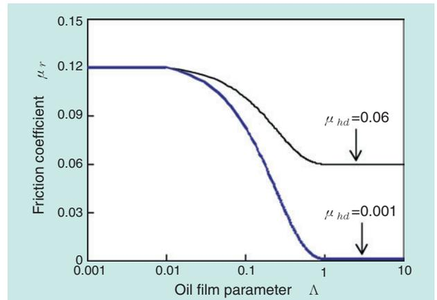
Fig. 3 Relationship between friction coefficient and oil film parameter
