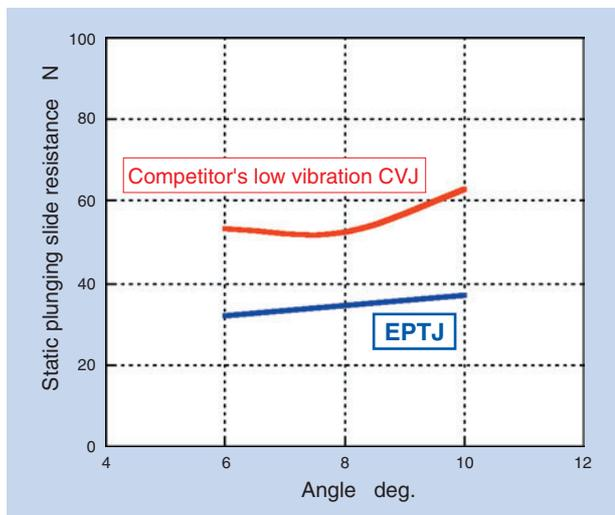
Fig. 4 Static plunging resistance vs operating angle under torque and stimulated vibration condition
