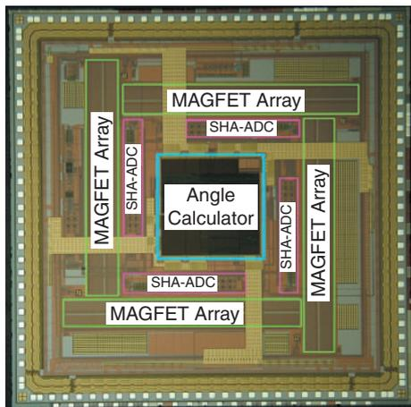
**Photo 1** Micrograph of a prototype chip
