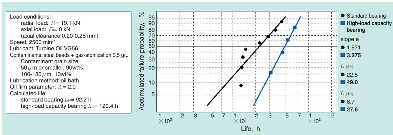
**Fig. 4** Life test results under contaminated lubrication
