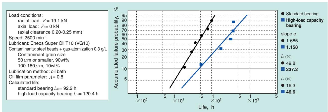
Fig. 6 Life test results under contaminated lubrication
