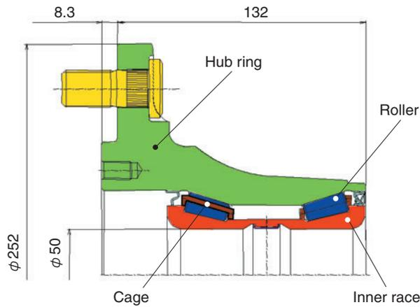
Fig. 1 Front non-driven GEN2 HUR structure
