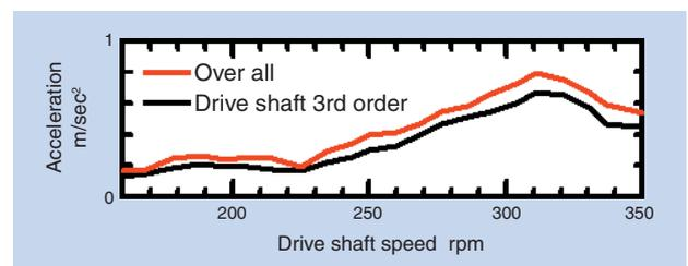
Fig. 2 Tracking result of fig.1 (c)
