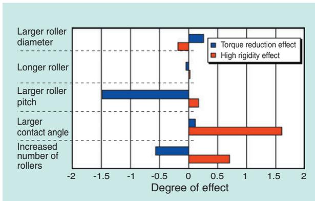
Fig. 11 Effect of internal design factors in torque and rigidity
