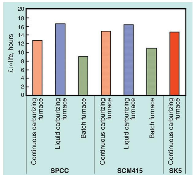
Fig. 2 Effect of race material and heat treatment furnace on bearing life
