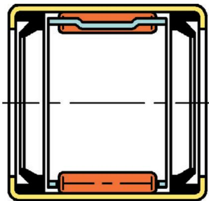
Fig. 2 Structure of drawn cup needle roller bearings for throttle bodies
