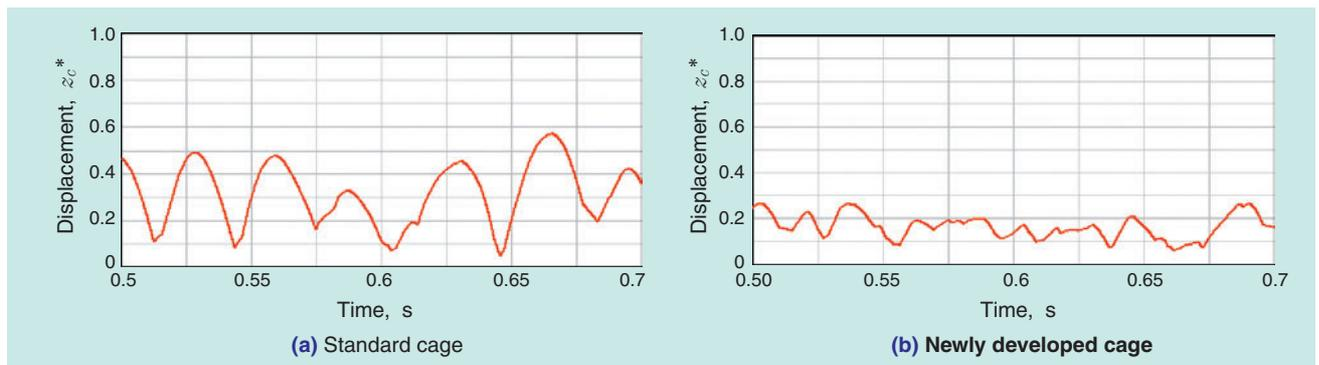
Fig. 11 Axial behavior of cage mass center
