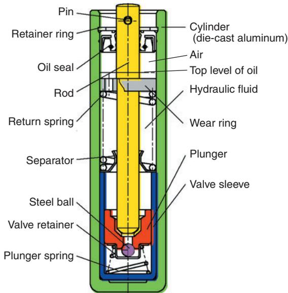
Fig. 3 Sectional view of Auto-tensioner
