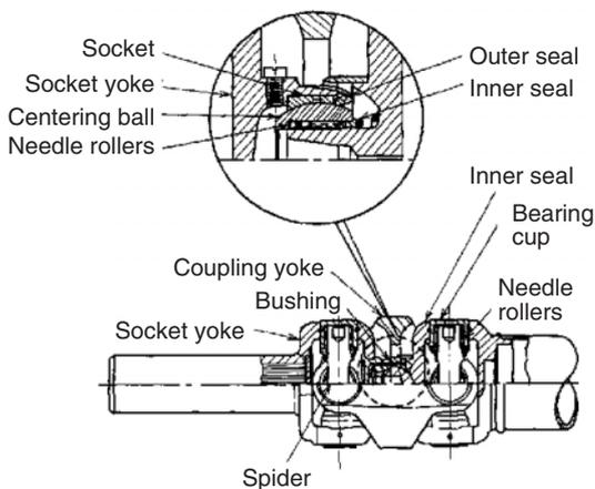
**Fig. 9** Double cardan joint
