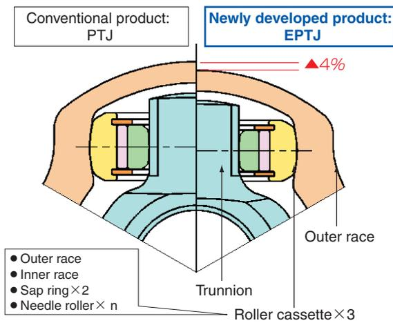
Fig. 1 Construction of PTJ and EPTJ
