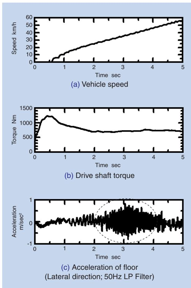
Fig. 1 Experimental Results of Shudder Vibration
