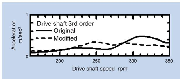
Fig. 8 Effect of engine mode on shudder vibration
