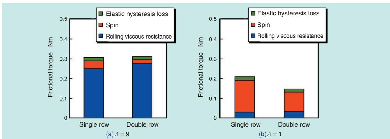
Fig. 15 Oil film parameter and factors of bearing frictional torque
