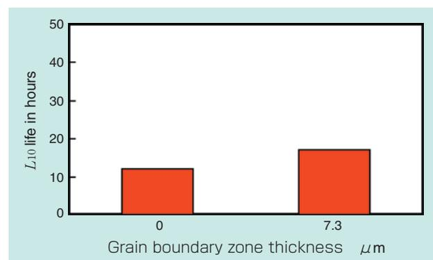
Fig. 5 Effect of race grain boundary oxidizing zone on bearing life
