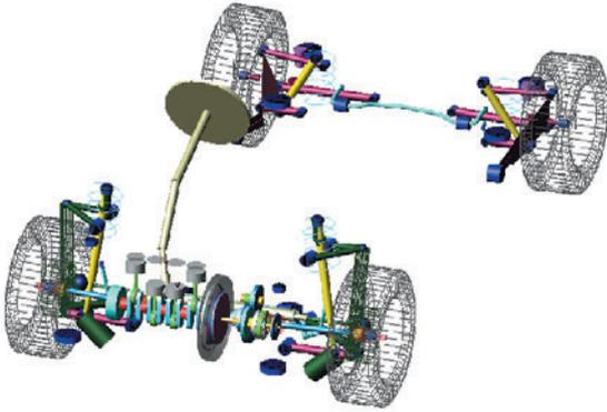
Fig. 3 Multi body Powertrain & Chassis model
