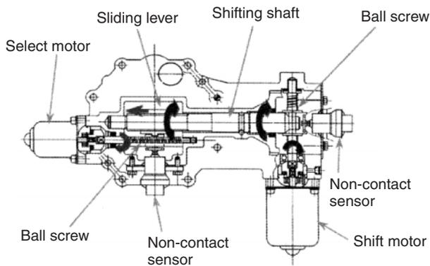
Fig. 1 Construction of gear shift actuator
