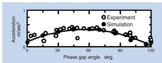
Fig. 12 Effect of CVJ phase gap on shudder vibration
