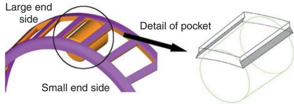
**Fig. 4** Geometrical shape of cage pocket
