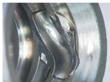
Photo 4 Appearance of deflector staking assembly
