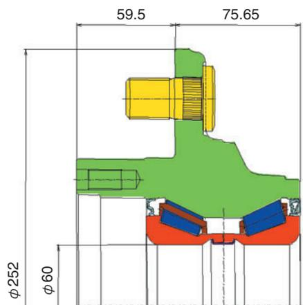
Fig. 2 Rear driven GEN2 HUR structure
