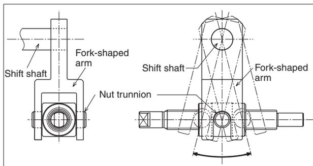
Fig. 2 Driving way of ball nut
