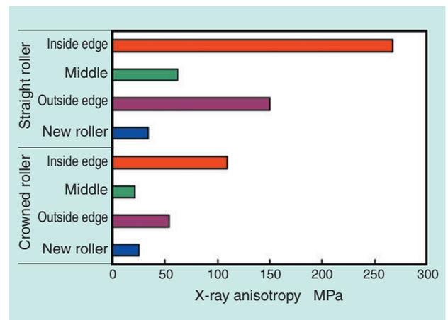
Fig. 9 X-ray anisotropy of rolling marks on races
