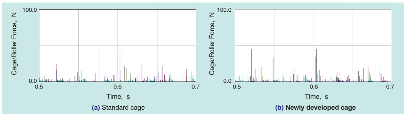
**Fig. 9** Cage/roller (rolling surface) interaction forces
