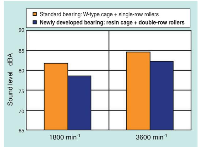
**Fig 13** Measurement result of sound level
