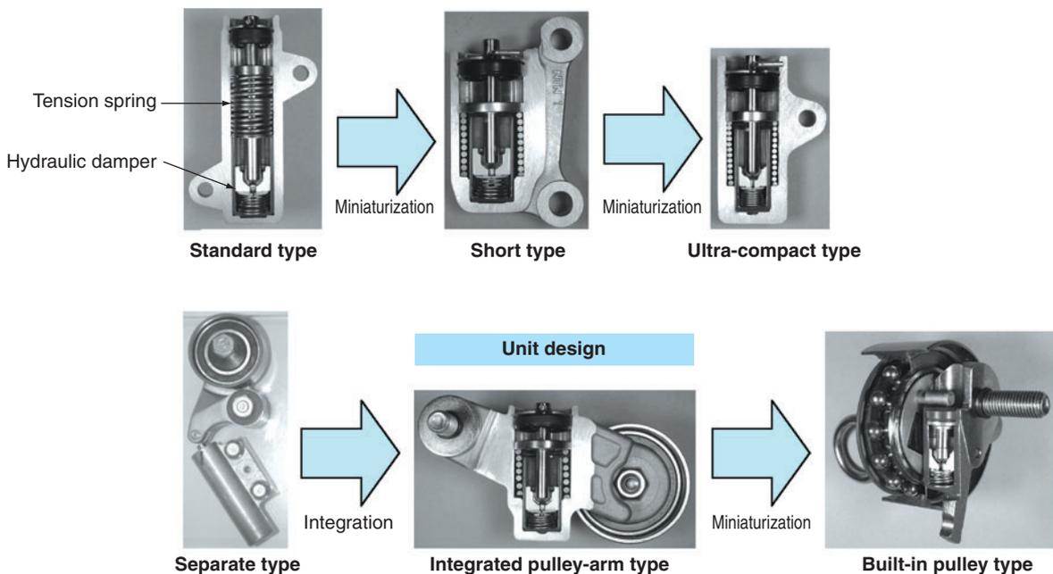
Fig. 4 Various Auto-tensioner's for timing belt
