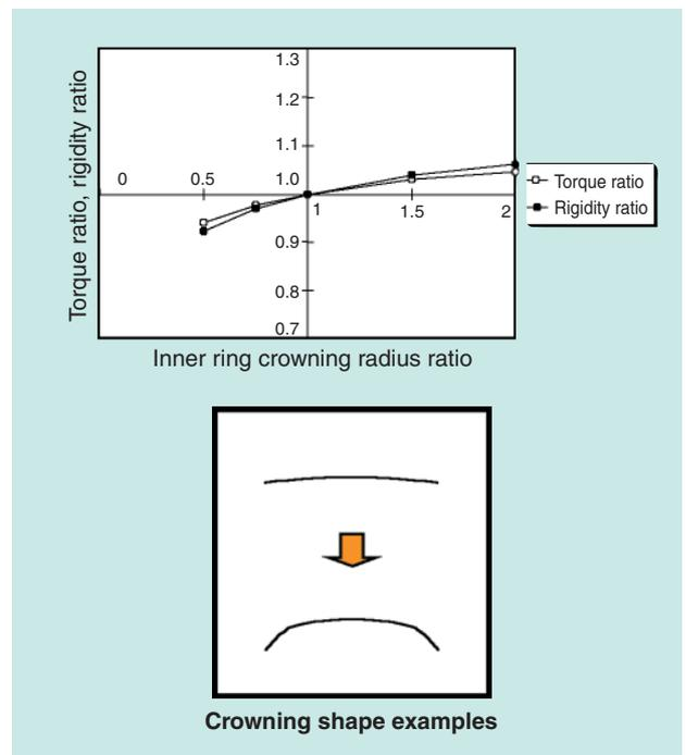
Fig. 13 Factors contributing to friction torque and rigidity of inner ring crowning
