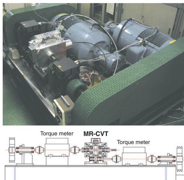
Fig. 6 Test rig for measuring transmission efficiency
