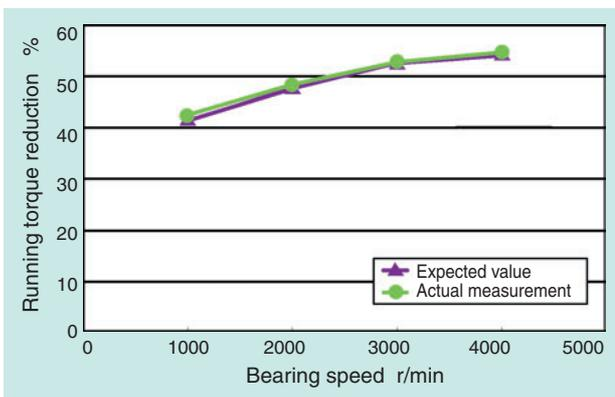
**Fig. 21** Relationship between speed and torque of low torque bearing
