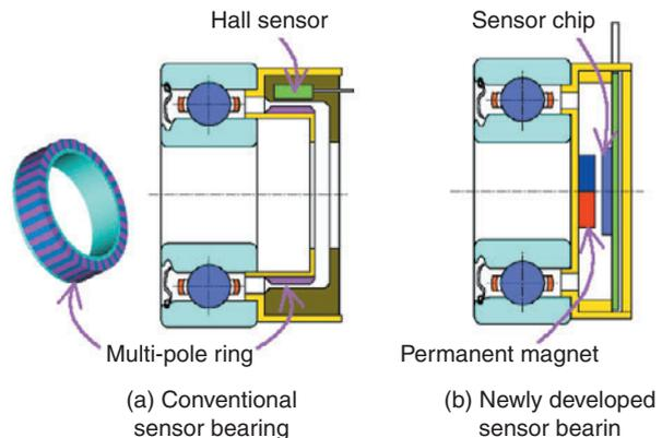
**Fig. 11** Cross section of sensor bearings
