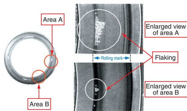
Photo 1 Raceway after life test
