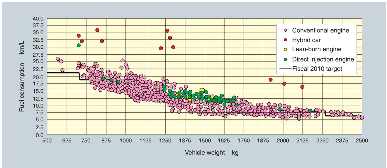
Fig.3 Fuel consumption on gasoline passenger cars (Home page of Ministry of Land, Infrastructure and Transport)
