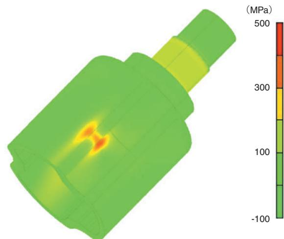
Fig. 5 FEM stress analysis for outer-race
