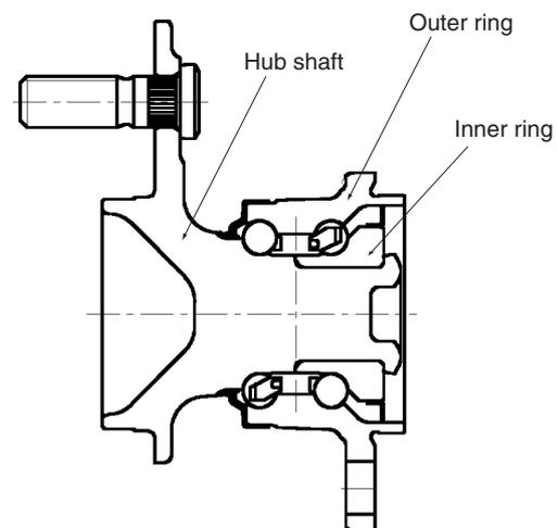
**Fig.1** Hub-Bearing original design
