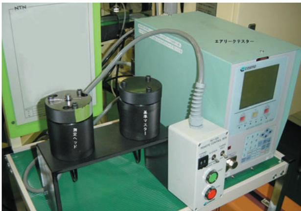
**Photo 1** Air leakage tester
