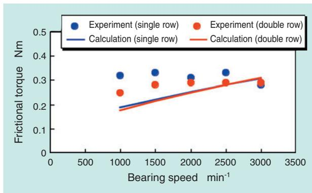
Fig. 14 Test and calculation results of bearing frictional torque with ISO VG 32 oil
