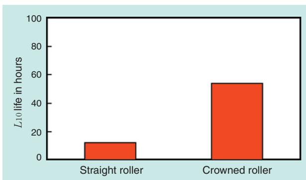
Fig. 7 Comparing bearing life with straight rollers and one with crowned rollers
