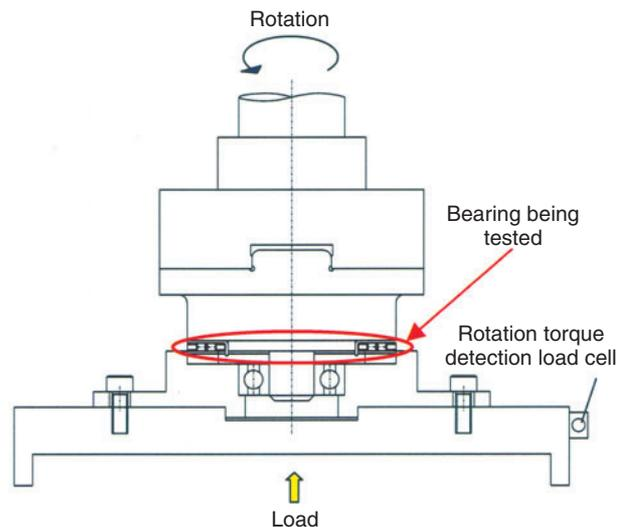
**Fig 5** NTN vertical type thrust bearing rotation torque test rig
