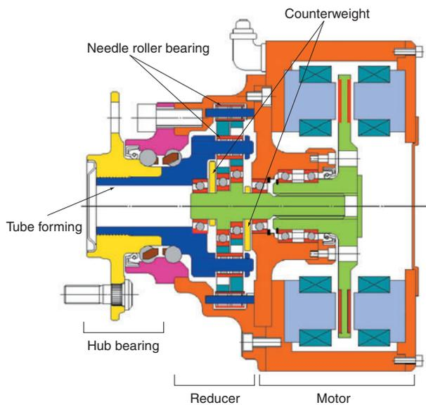
Fig. 1 Schematic of axle unit
