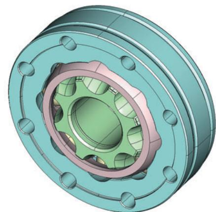
Fig. 4 HEBJ disc type design
