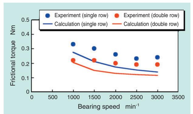
Fig. 13 Test and calculation results of bearing frictional torque with ISO VG 2 oil
