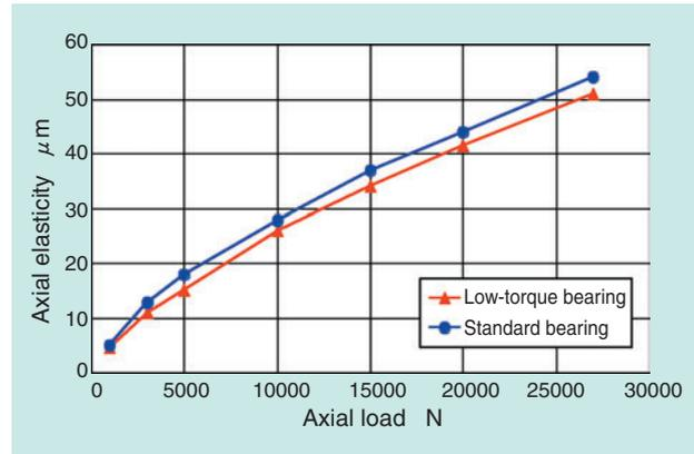
**Fig. 22** Deformation of axial direction
