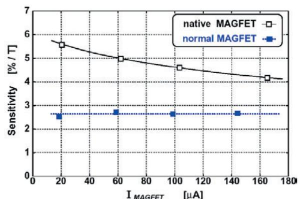
Fig. 9 Magnetic sensitivity of the MAGFETs ( $I_{MAGFET}$ : bias current in a MAGFET)
