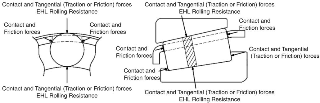
Fig. 1 Considered interaction forces in this dynamic analysis
