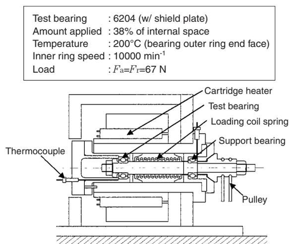
Fig. 3 Grease life test rig
