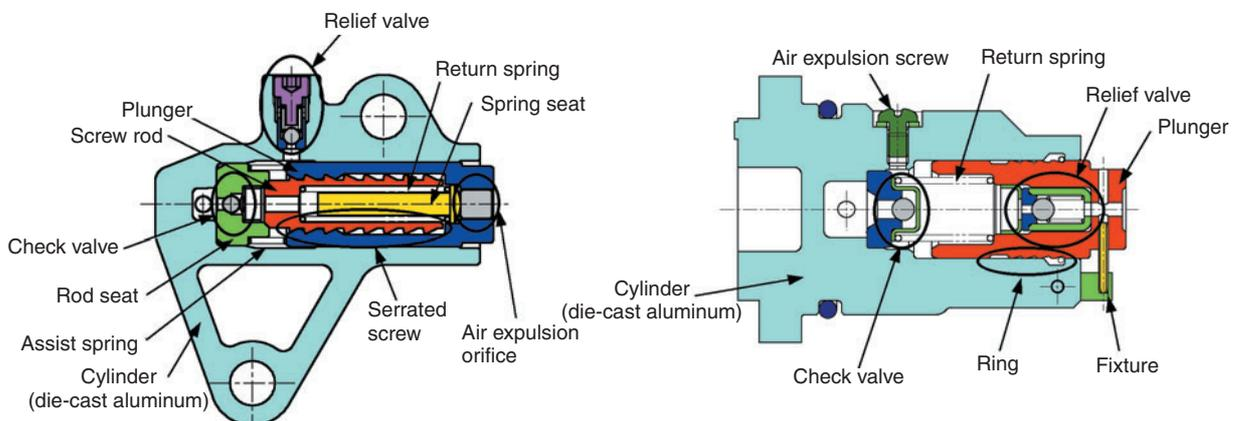
Fig. 8 Various Auto-tensioner for timing chain
