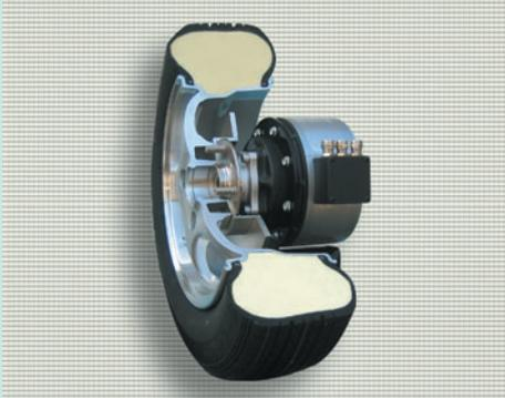
NTN has been developing the in-wheel type integrated motor axle unit for electric vehicles. The unit accomplishes compact size and light weight by integrating a hub bearing, a cycloid reducer and a high-speed motor, realizing least increase in the unsprung mass of in-wheel motor vehicles. This paper introduces the design concept and basic performance of the unit.
