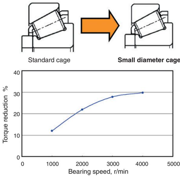
Fig. 17 Relationship between speed and torque reduce percentage of bearing with small diameter cage
