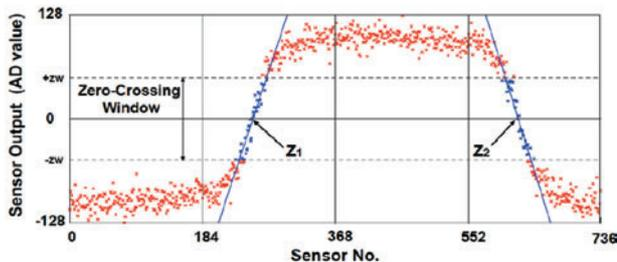
Fig. 5 Output signal of the sensor arrays
