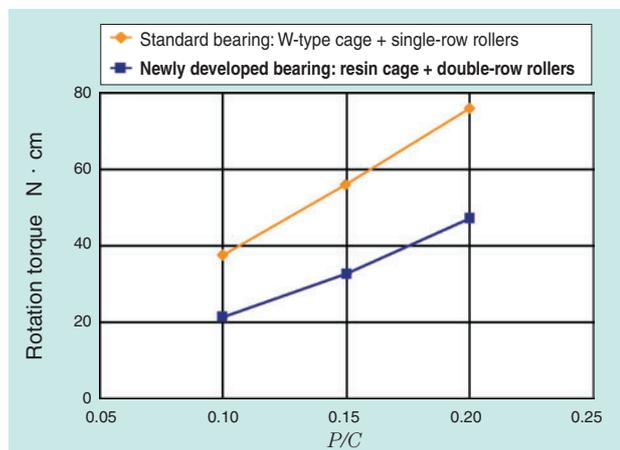
Fig 12 Measurement result of rotation torque
