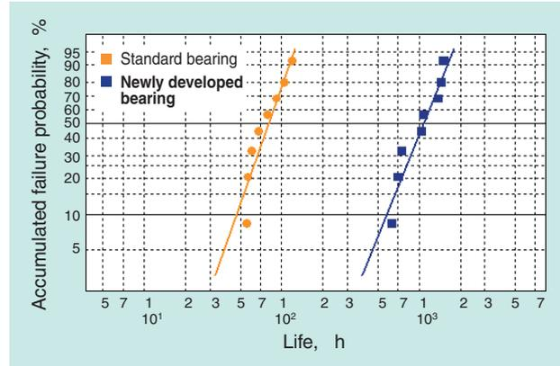
**Fig 3** Result of life test condition 1 with misalignment for car air conditioners
