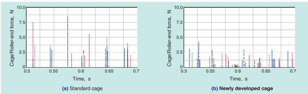
Fig. 14 Cage/roller large end interaction forces
