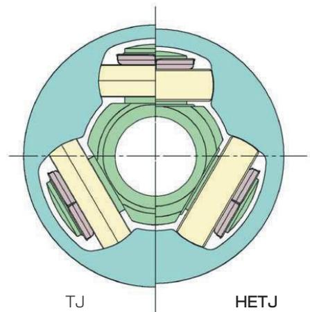
Fig. 7 Comparison of structure between TJ and HETJ
