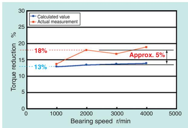
**Fig. 16** Relationship between torque and torque reduce percentage
