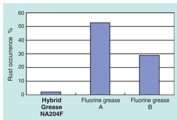
**Fig. 6** Rust prevention ability of greases
