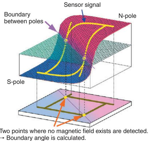
Fig. 6 Detection of the Zero-Line
