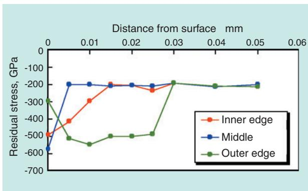
Fig. 6 Compressive residual stress in a race after test
