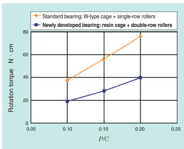
Fig 6 Measurement result of rotation torque
