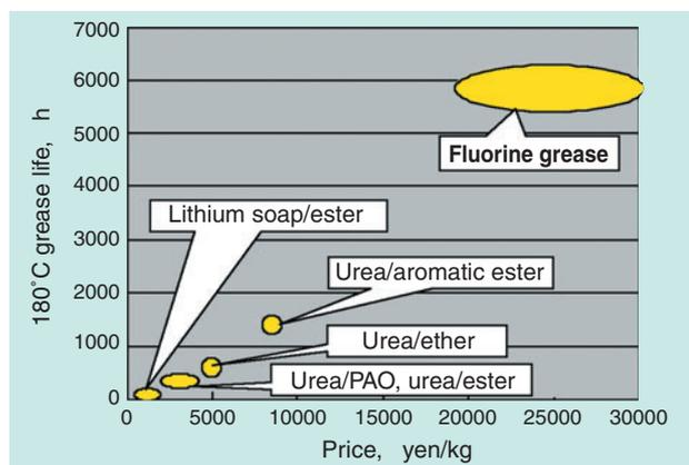
Fig. 1 Cost and high temperature life of greases
