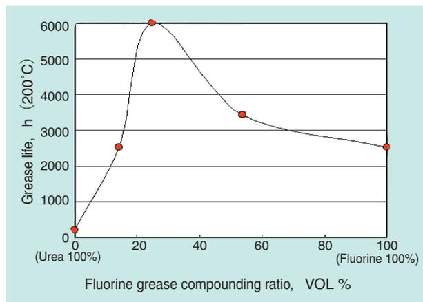
Fig. 2 High temperature life of Hybrid Grease
