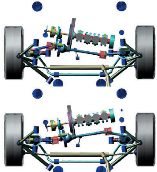
Fig. 7 Lateral engine mode shape (12.33Hz) of modified model
