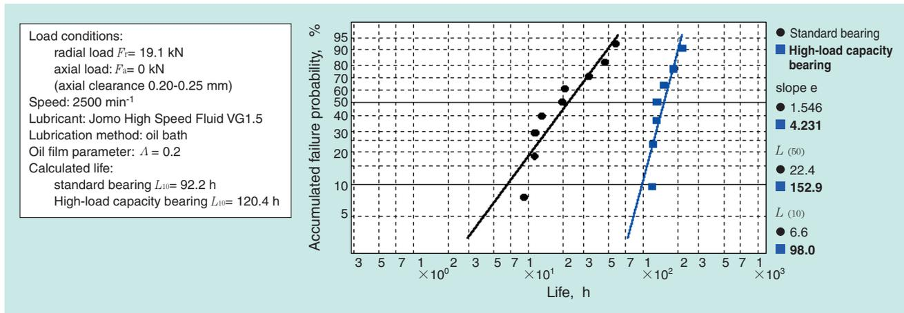
**Fig. 3** Life test results under clean lubrication
