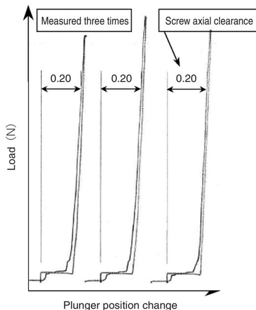
**Fig. 10** Static characteristic of 'No-back' mechanism
