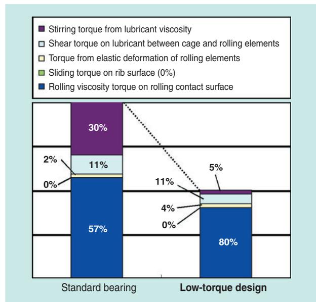
**Fig. 23** Analysis of torque reduction
