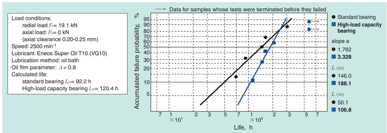
Fig. 5 Life test results under clean lubrication
