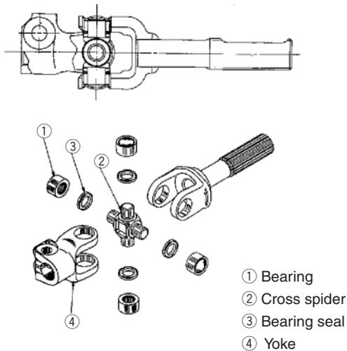
**Fig. 8** Cross joint (Cardan joint)
