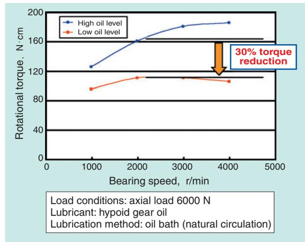
Fig. 8 Torque of tapered roller bearing used for pinion shaft support in near axle differential
