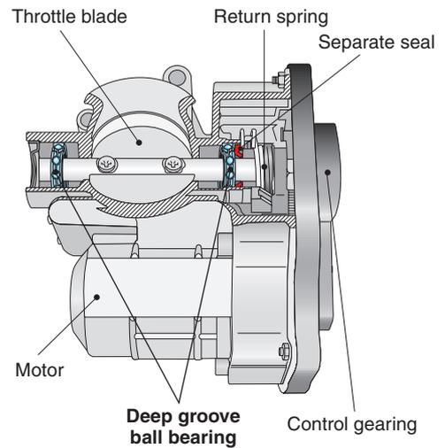
Deep groove ball bearing application example
