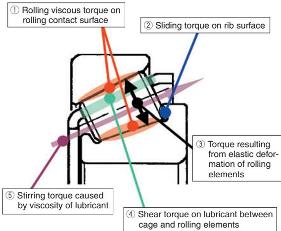
Fig. 7 Torque factor of tapered roller bearing
