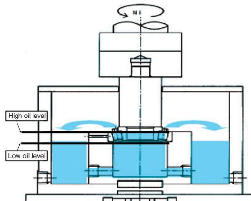
Fig. 9 Torque measurement method
