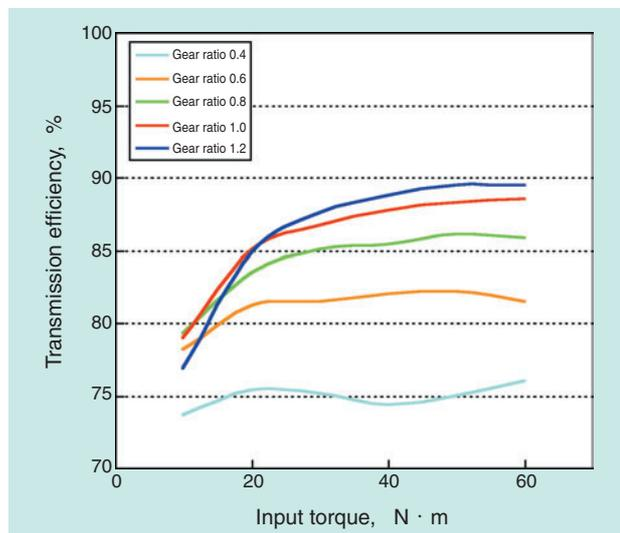
Fig. 9 Input torque and transmission efficiency (4000min<sup>-1</sup>)
