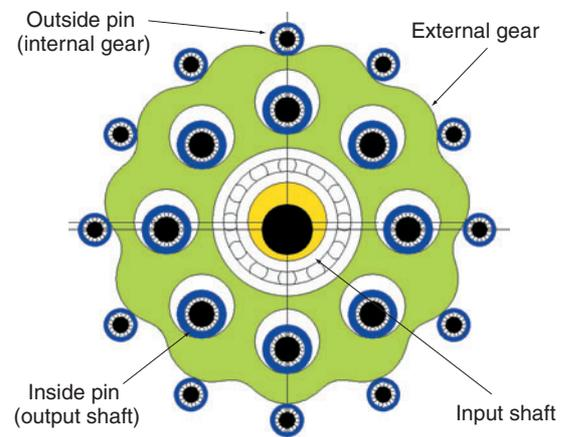
Fig. 4 Basic structure of reducer
