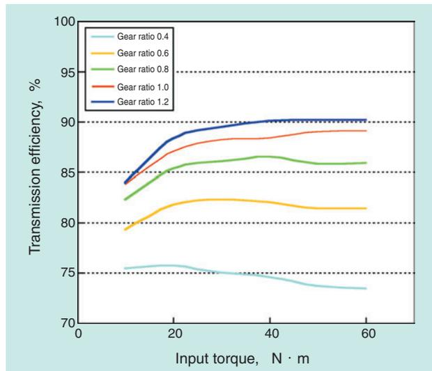
Fig. 8 Input torque and transmission efficiency (2000min<sup>-1</sup>)
