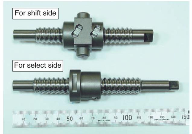
Photo 2 Ball screw for AMT
