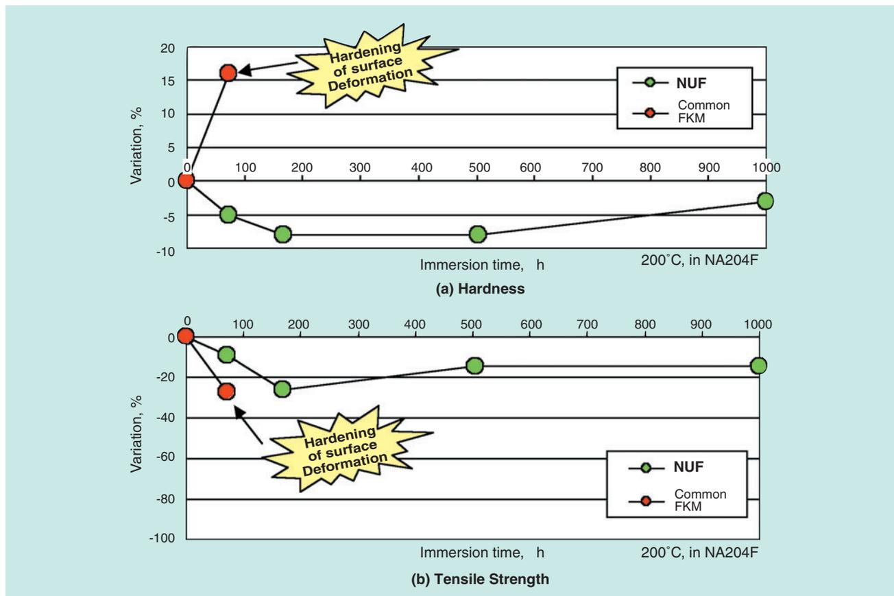
**Fig. 8** Deterioration of fluorinated rubbers dipped into Hybrid Grease at 200°C
