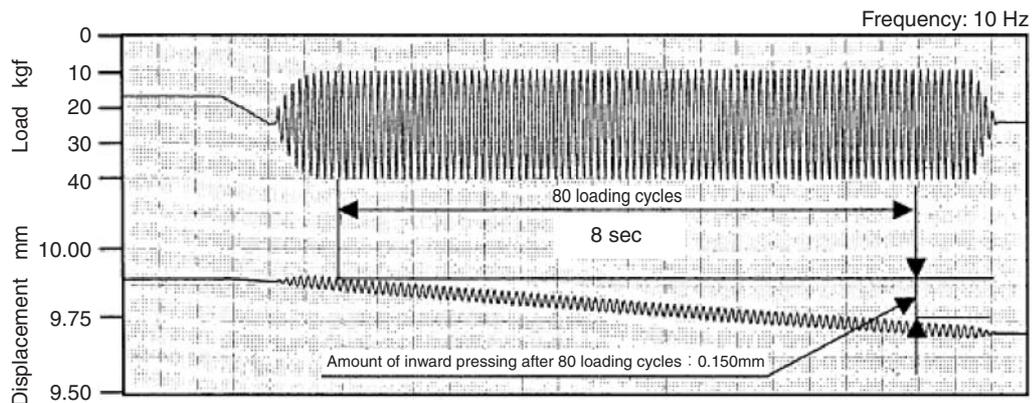
Fig. 11 Dynamic characteristic of screw plunger
