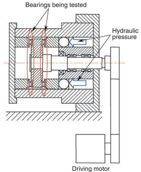
Fig. 1 NTN thrust needle roller bearing life test rig
