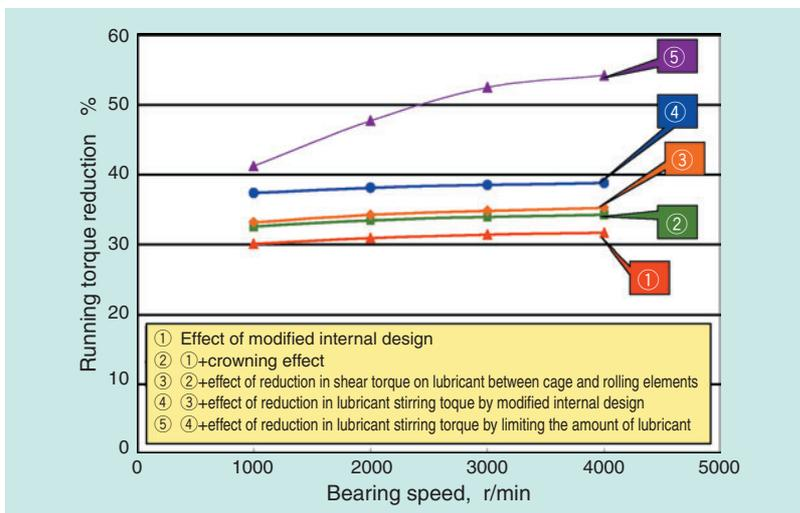
Fig. 19 Relationship between speed and torque of each torque reduction factors
