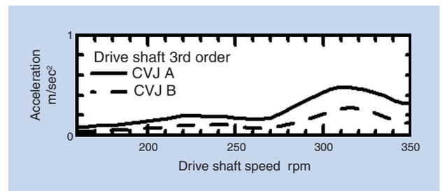
Fig. 9 Effect of CVJ on shudder vibration (Induced Thrust CVJ A > CVJ B)
