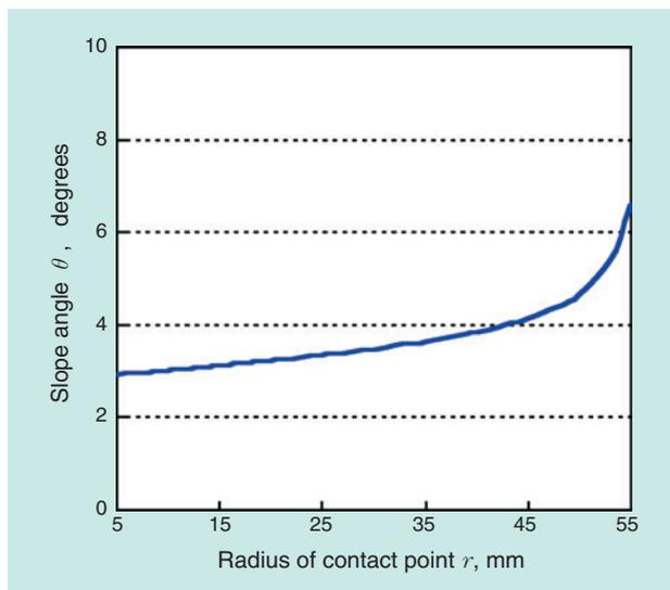
Fig. 5 Relation between radius of contact point and slope angle of V-pulley
