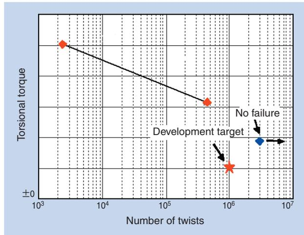
Fig. 6 Torsional fatigue strength
