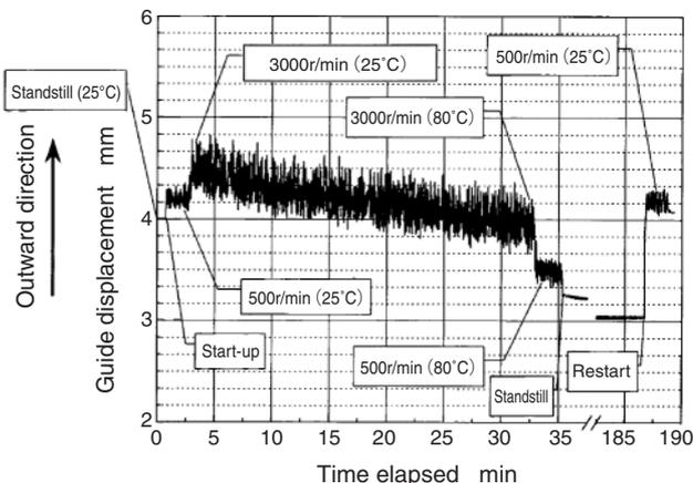
**Fig. 9** Plunger position during engine operation
