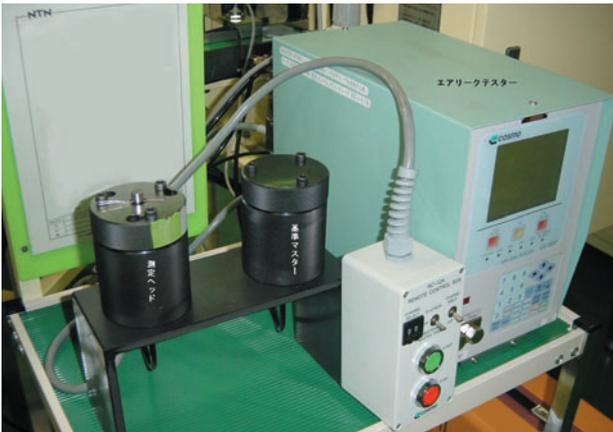
**Photo 1** Air leakage tester
