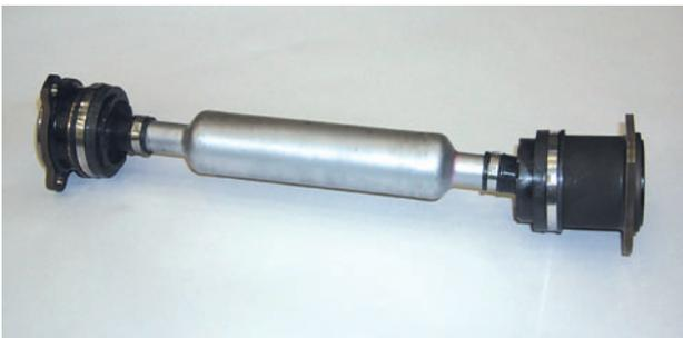
Photo 1 Example of Propeller shaft. (2 joint design)
