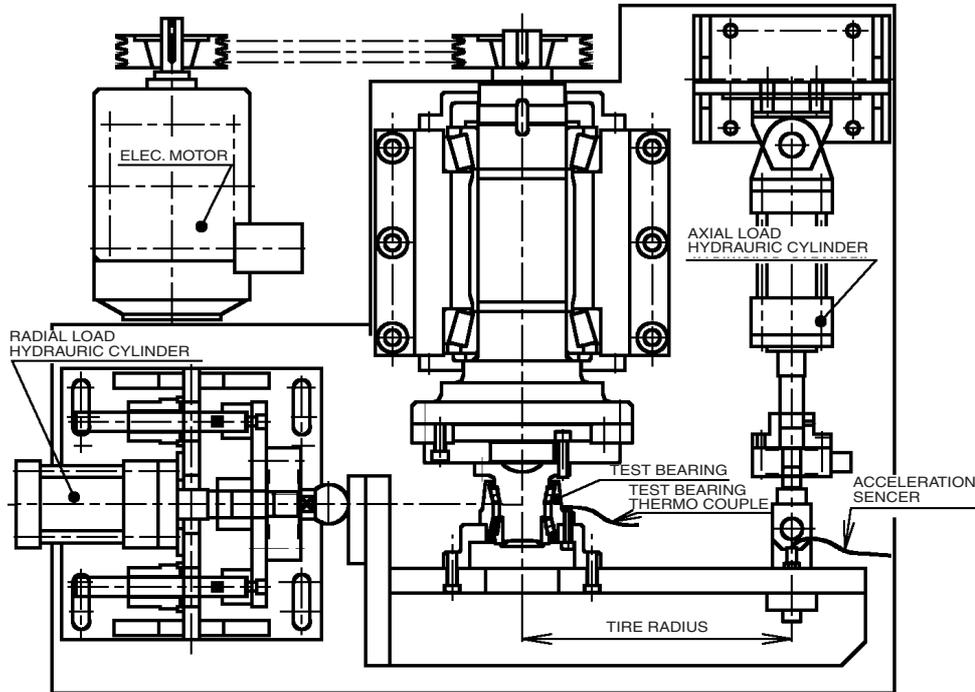
Fig. 5 Test machine structure
