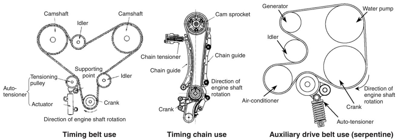
Fig. 1 Layout of Auto-tensioner (example)
