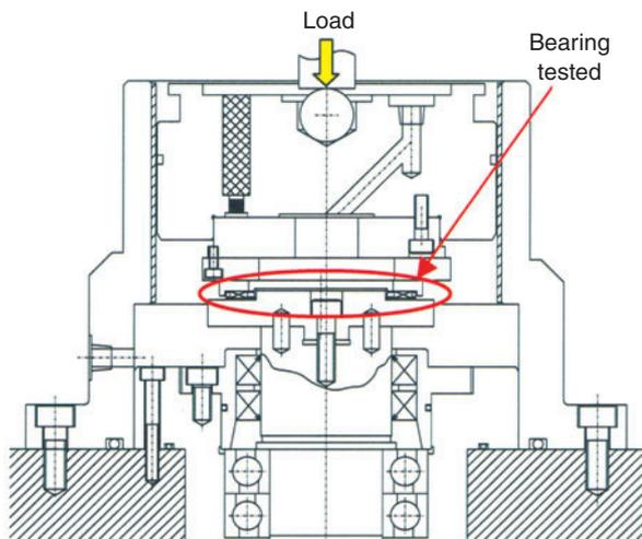
Fig 11 NTN vertical type thrust bearing test rig for eccentricity rotation
