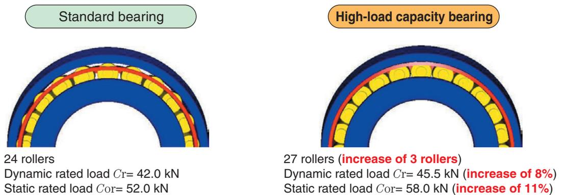
Fig. 2 Example of bearing design (size :  $\phi 45 \times \phi 81 \times 16$ )
