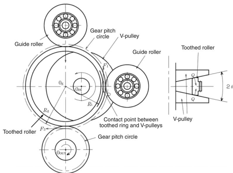
Fig. 2 Basic mechanism of MR-CVT
