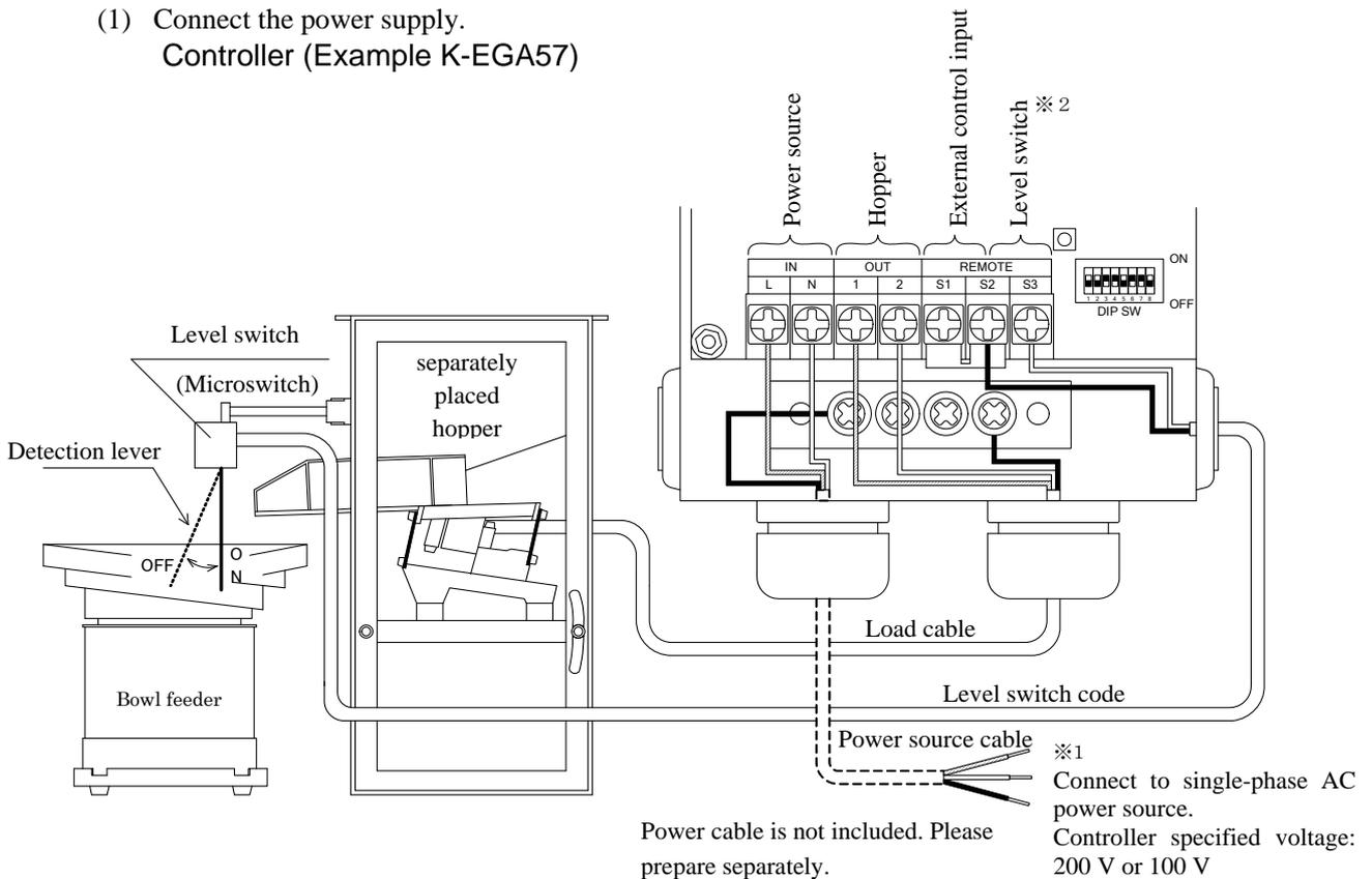
※1 In the case of three-phase power supply, use any two phases out of three. Do not use the balance one phase.
