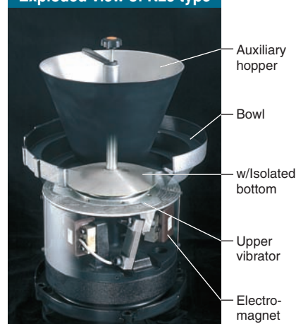
Exploded view of N25 type
