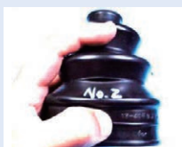
Cracks develop due to repeated flexing during rotation, leading to fractures
