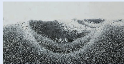
Cross-section of region with electrical corrosion
