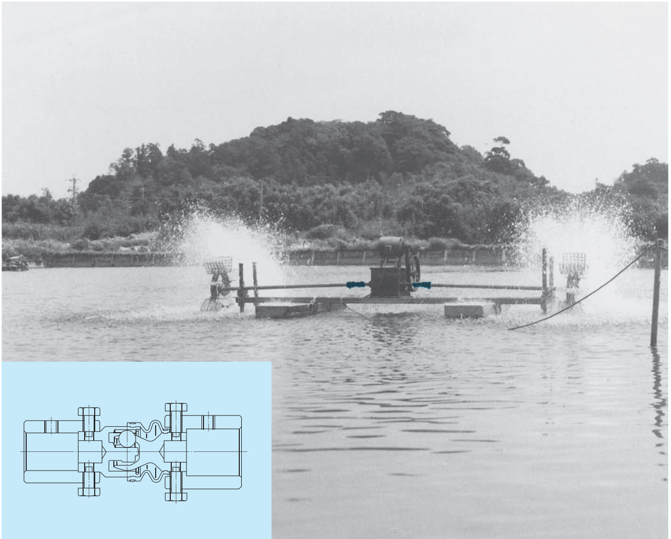
▲Driving area of a water wheel in an eel farm.
