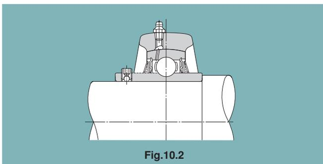
each other. UK type bearing can't support axial load.
