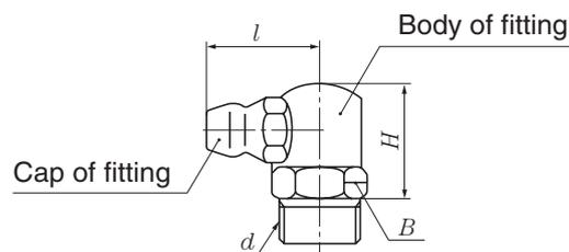
**Table 9.5 Grease fitting types available for bearing units**
