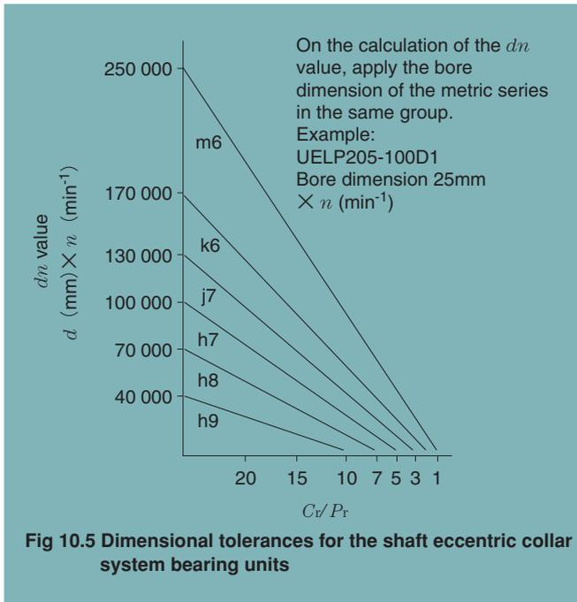
**Fig 10.5 Dimensional tolerances for the shaft eccentric collar system bearing units**
