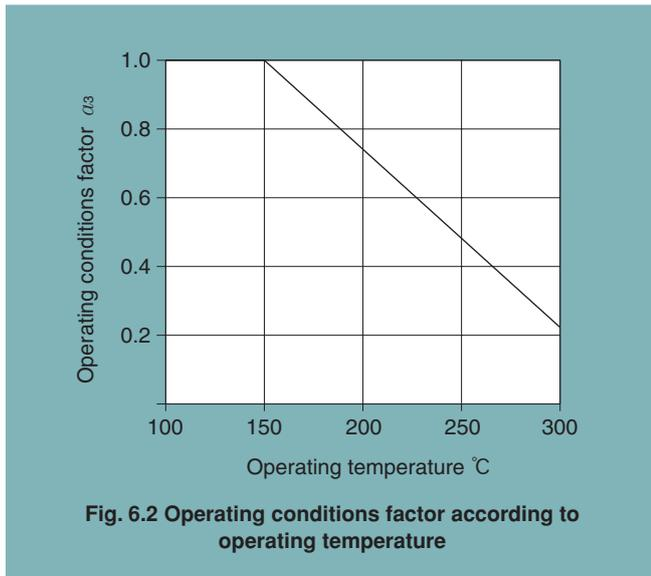
**Fig. 6.2 Operating conditions factor according to operating temperature**
