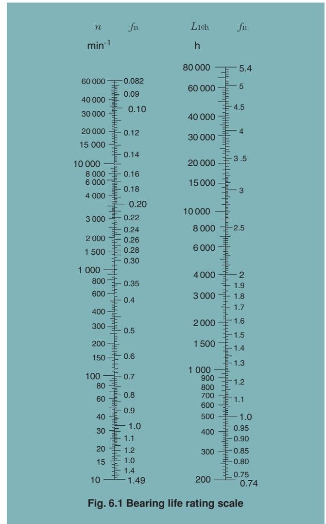
Fig. 6.1 Bearing life rating scale
