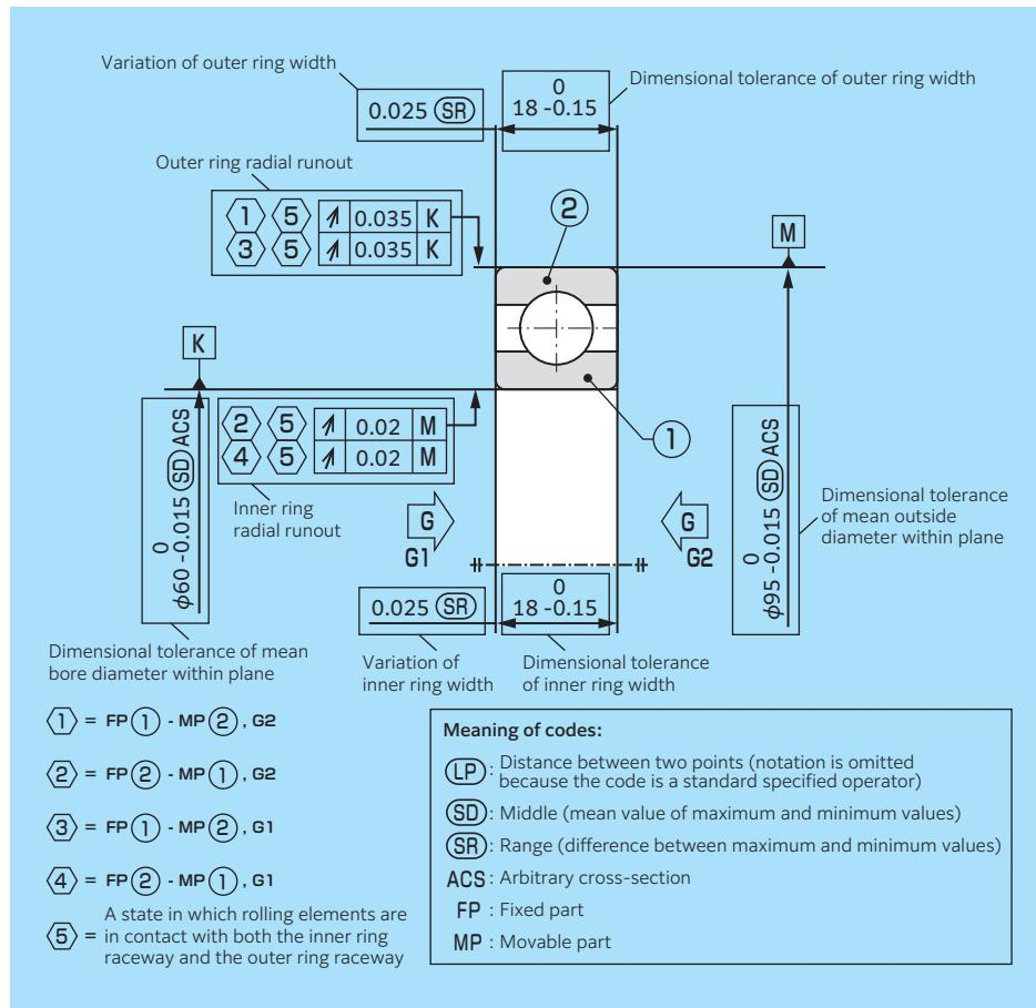
Fig. 6.3 Example of bearing drawing applying GPS
