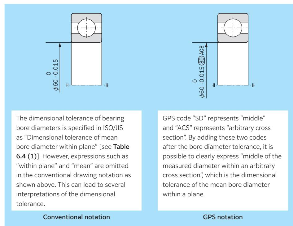
**Fig. 6.2** Notation example of bearing bore diameter tolerance
