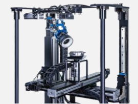
An appearance inspection system utilizing the “i-WRIST,” Wrist Joint Module
