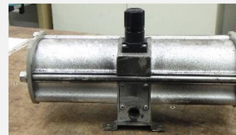
Visualization of air consumption per process by installation of an air flow meter revealed an air leak in the pressure booster tank, and countermeasures were taken (Kuwana Works)
