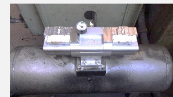
Visualization of air consumption per process by installation of an air flow meter revealed an air leak in the pressure booster tank, and countermeasures were taken (Kuwana Works)
