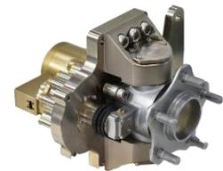
“Ra-sHUB” Hub Bearings with Steering Function for Rear Wheels
