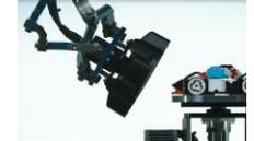
i-WRIST™ equipped with camera enables automation of visual inspection conducted by human
