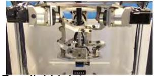
Parallel Link type High Speed Angle Control Equipment
