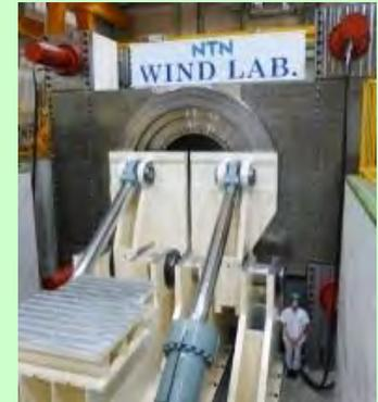
Testing Machine for Wind Turbine
