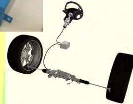
Steering System for Steer-by-Wire
