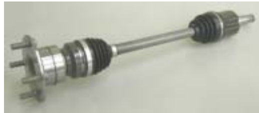
V-series 4th generation hub joints
