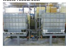
At NTN Bearing Mfg. Canada (CMF), a water circulation system was installed to reduce the amount of water used for tumblers. The company succeeded in reducing annual water use by 1,920 kl and halving the amount of wastewater.  $\Rightarrow p57$
