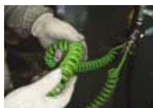
Inspecting for air leaks
