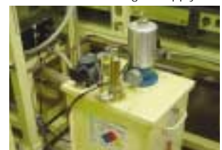
New rust inhibiting oil supply unit
