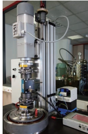
Fig. 12 Starting test measurement test bench
