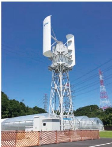
図13 10kW垂直軸風車 10kW vertical axis wind turbine
