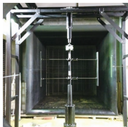
図16 垂直軸風車の風洞実験 (三重大学大形風洞) Wind tunnel experiment of vertical axis wind turbine (Mie University Large Wind Tunnel)
