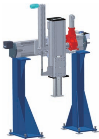
図14 高負荷容量昇降軸 High load capacity linear module for lifting axis
