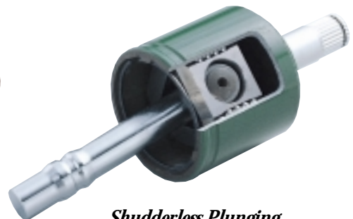
Shudderless Plunging Constant Velocity Joint (BTJ)
