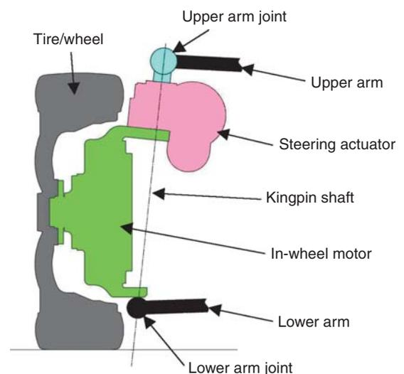
**Fig. 3** Suspension layout
